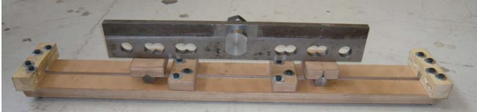
Figure 108, Altered upper support flange.
