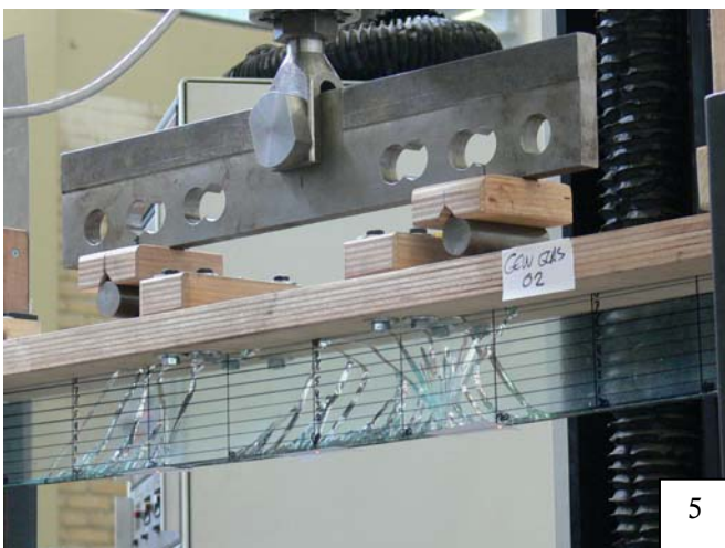
Figure 110, Test 2 on 6 different stages of the test. First crack is visible on picture 2. Further cracks are visible on photos 3 and 4. Total failure has occurred on photo 5. The final result of test 2 is visible on photo 6.
