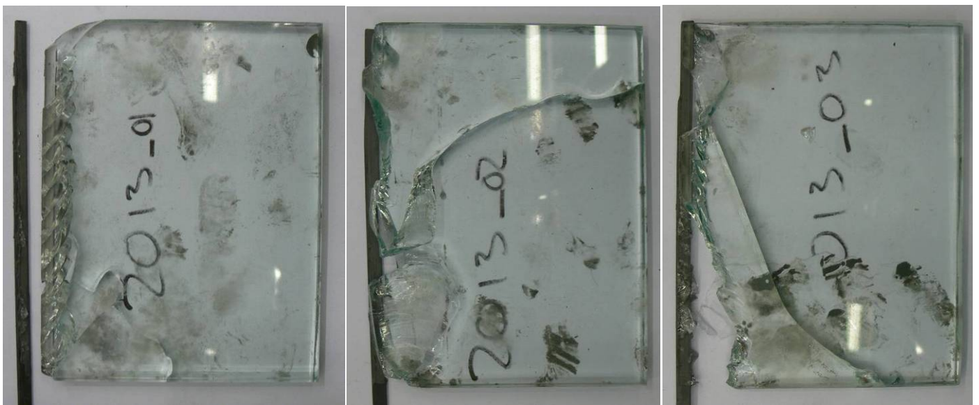
Figure 33, Specimens 2013_01, 2013_02 and 2013_03 after the test
