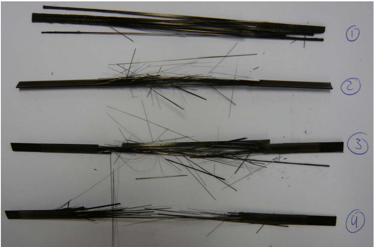
Figure 5, Flat specimens 1 to 4. Specimen 1 failed due to clamping force. The tests of specimens 2 to 4 resulted in higher ultimate tensile stresses
