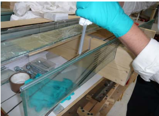
b: Application of adhesive at specimen 3
