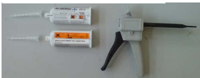
e: Ready-mix nozzle, adhesive cartridges of both adhesives and glue squirt.
