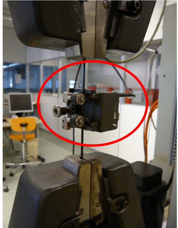
Figure 3, Photo of test set-up with round carbon fiber specimen. The device in the middle of the picture (circled in red) is the Zwick extensometer
