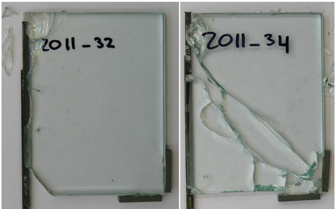
Figure 88, Above: specimen 2011_32 at different moments during the test, corresponding to the moments in Error! Reference source not found.. Picture 'f' was taken after total failure. Below: Specimen 2011_32 and 2011_34 after the test.
