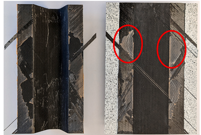
Fig. 13. Control1 Specimen Fracture Surface.
