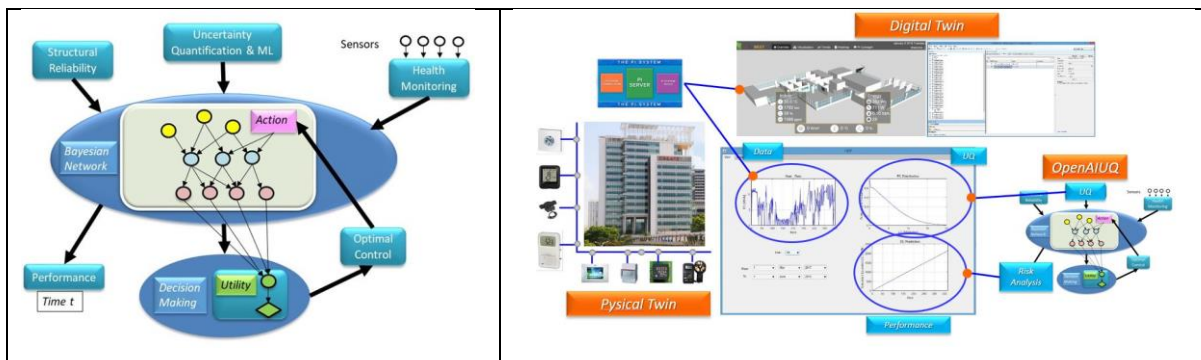
Figure 1. (a): Risk-Informed Digital Twin (RDT), computational platform, (b): implementation of the RDT into a smart building in CREATE Office, Singapore
