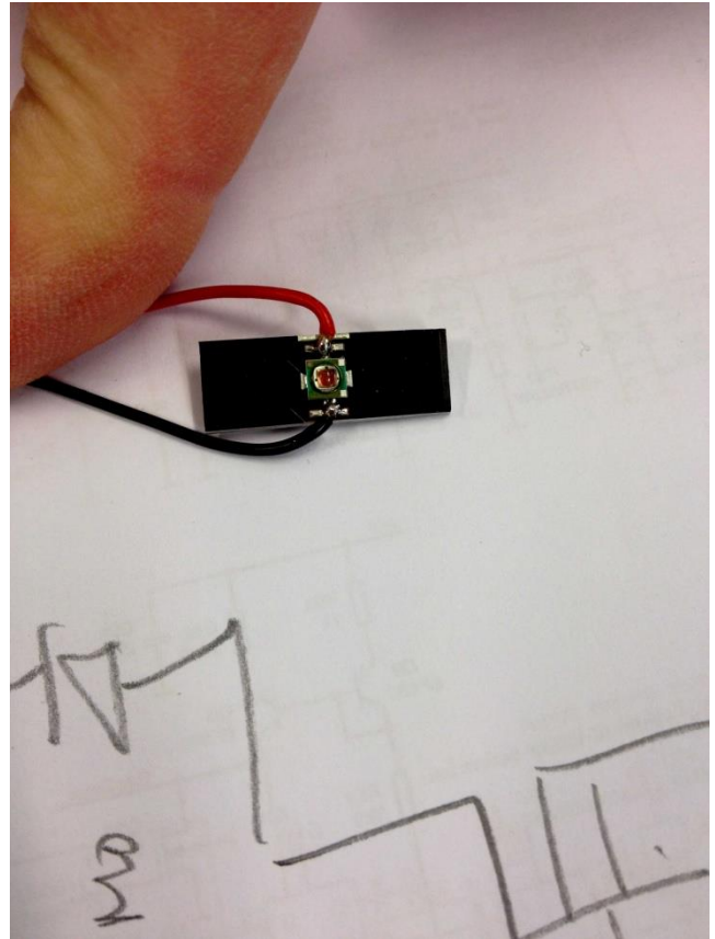
LED from CREE mounted in aluminium plate
