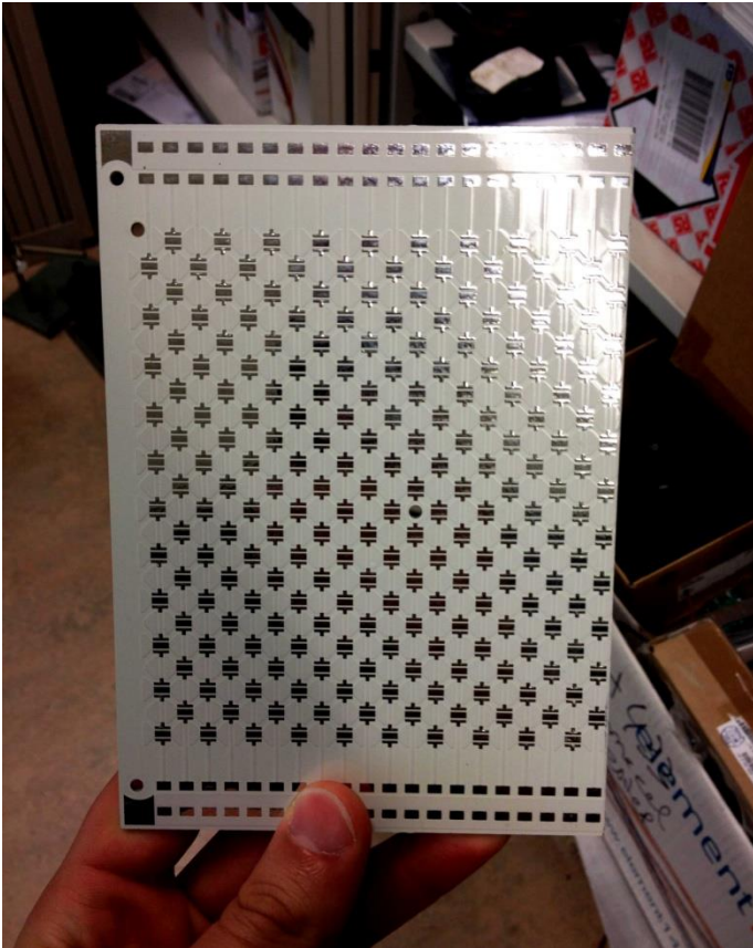
PCB made of aluminium due to the high temperature emitted by the LEDs
