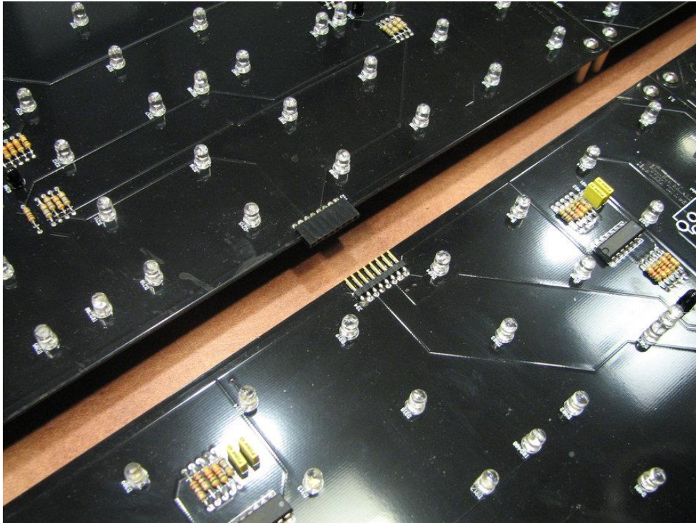
Closer view of the panel with the connection chips and the motion sensors ( http://shop.evilmadscientist.com/productsmenu/majors/46 )
