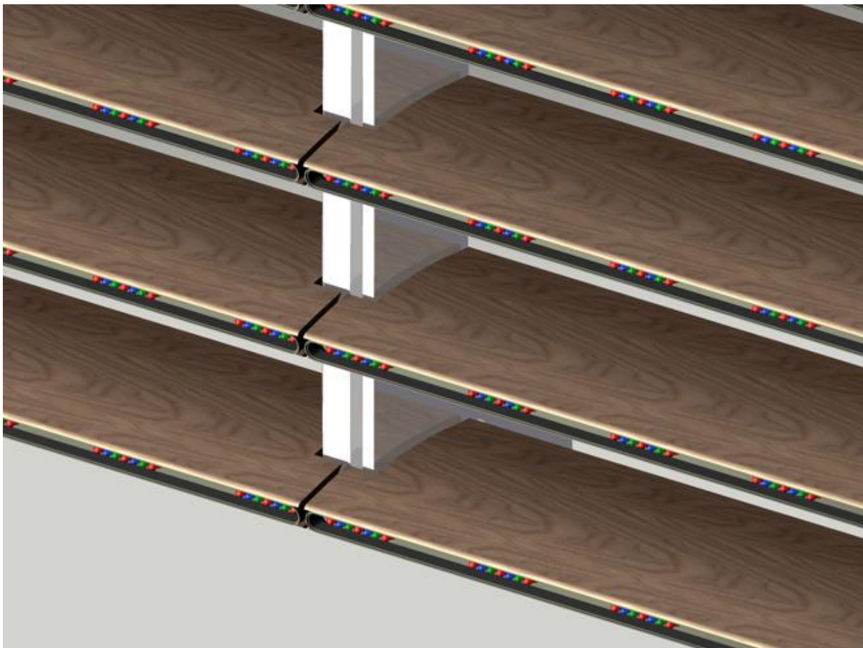
Closer view of the system with LEDs integrated on the front edge ( http://www.louvreled.com/ )
