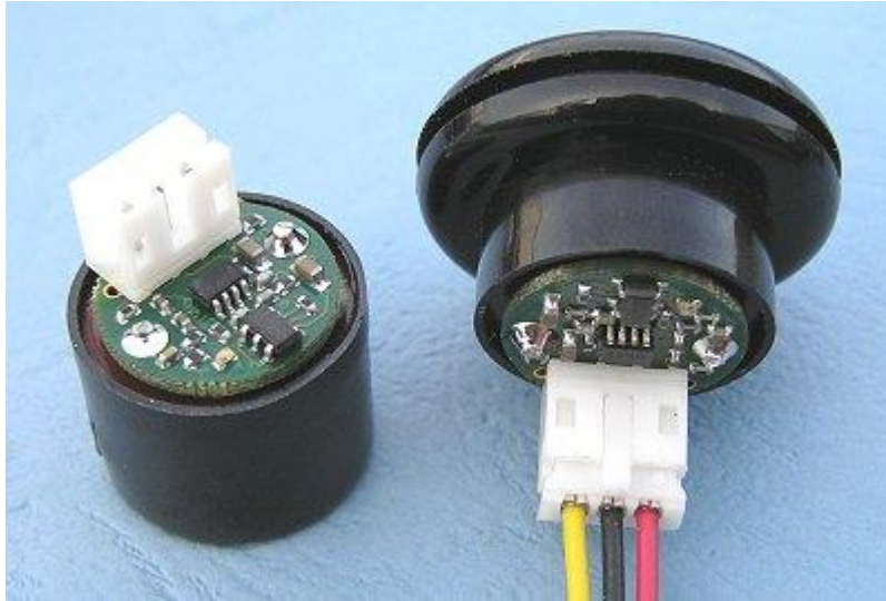
SRF01 Ultrasonic range finder with dimensions which can fit in a LED Strip ( http://www.robot-electronics.co.uk/ )
