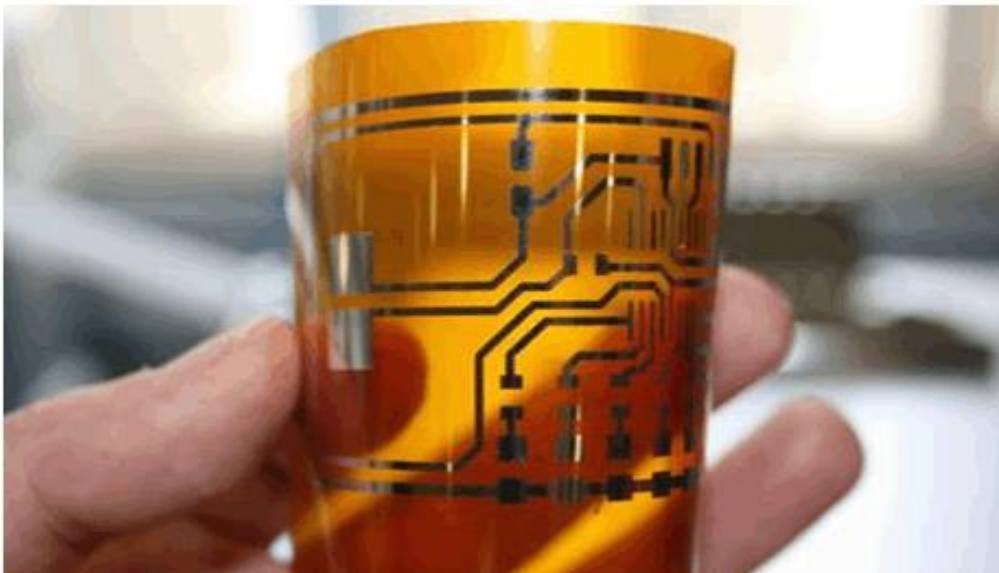
A flexible circuit by printed inject ( http://articles.ides.com/design/2010/plastic-electronics.asp )
