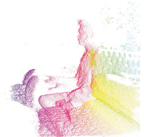
figure 55 IR point cloud of Kinect v2
