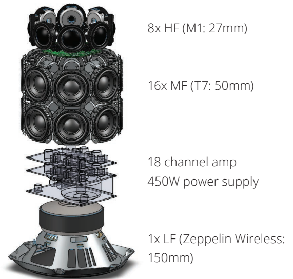
figure 20 Preliminary configuration for the intelligent concept speaker
