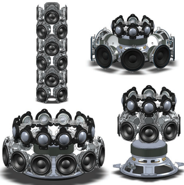
figure 19 Different configurations with an omnidirectional coverage
