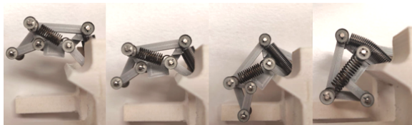
Figure 1-13: The resulting motion of the adaptive grip mechanism (with spring set 1).
