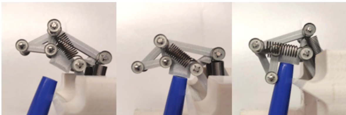
Figure C-7: The resulting motion of the adaptive grip mechanism when the proximal phalanx is obstructed (with spring set 1).
