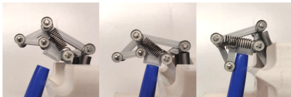
Figure 1-14: The resulting motion of the adaptive grip mechanism when the proximal phalanx is obstructed (with spring set 1).
