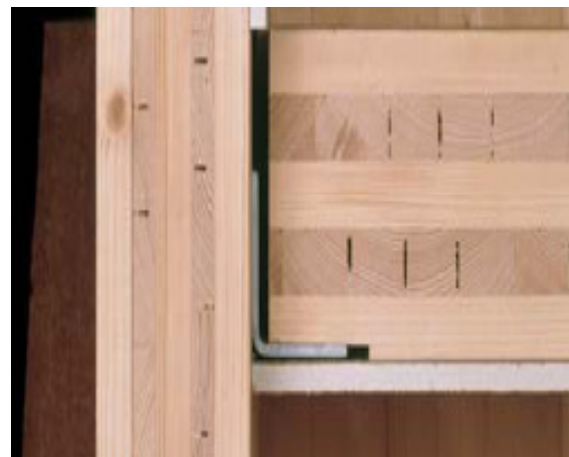
Figure 3.17 Balloon frame method Source: Informationsdienst Holz
