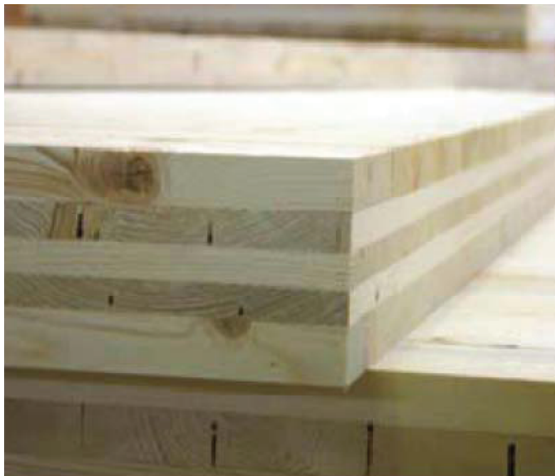
Figure 3.1 Cross laminated timber panel Source: Finnforest
