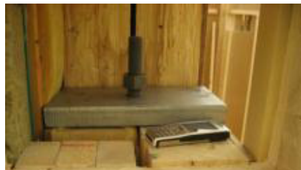
Figure 4.18 Stabilizing tie rod Source: Linnaeus University
