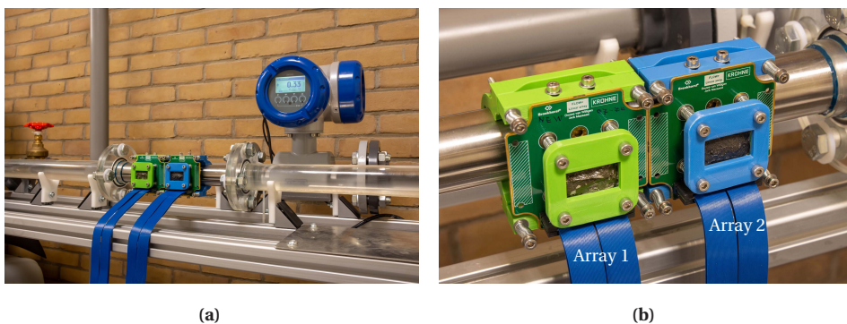
Figure 5.1: Custom-made flow loop to perform ultrasonic clamp-on flow measurements with the fabricated prototype arrays. Gravity was used to drive flow from left to right through the stainless steel pipe section on which the arrays were installed. A close-up picture (b) shows the custom-made 3D-printed green and blue frames of the prototype arrays. They were designed with a system of screws and springs to achieve good mechanical coupling of the array with the coupling piece (inner 4 screws), and of the coupling piece with the pipe wall (outer 4 screws).
