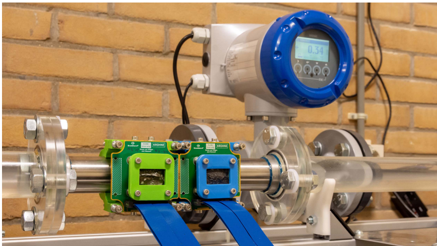
Figure 6.14: Array transducers mounted onto a steel pipe section in the flow loop, with the reference flow meter in the back.
