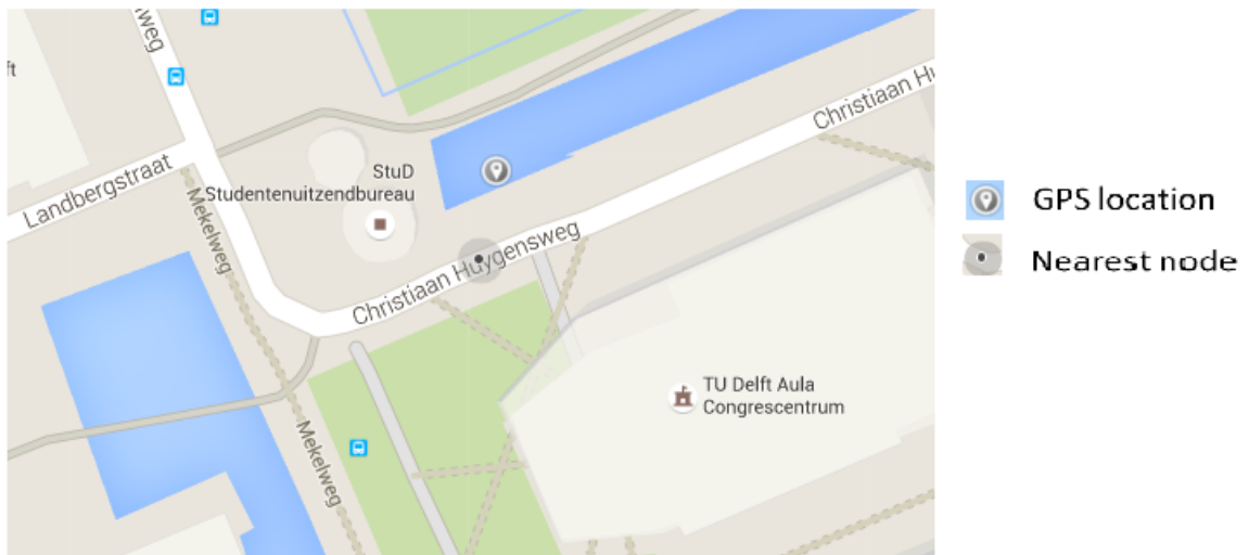
Figure 5.2, mapping GPS location (in the water) to the nearest node.
