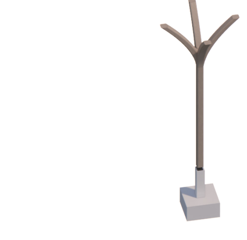
Secondary Columns + Towards the end as the new built, columns branch out into four, to reduce dependency on existing brick cavity walls.
