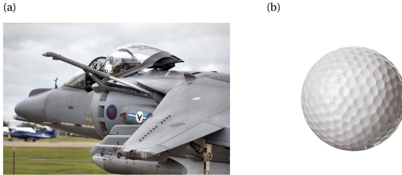
Figure 1.3: (a) Vortex generators on the wing suction side of a *Harrier II*. (b) Dimples on a golf ball.
