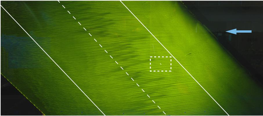
Figure 3.6: Same notation of figure 3.4.  $\alpha = 3^\circ$ . Cylindrical roughness elements ( $d_r = 2.8$  mm and  $k_r = 10$   $\mu$  m) installed at  $x/c = 0.025$  spaced 9 mm.
