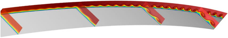
Figure 1.7: Streamwise evolution (from left to right) of primary CFVs. Contours of streamwise velocity (re-adapted from Tempelmann *et al.* [121]).
