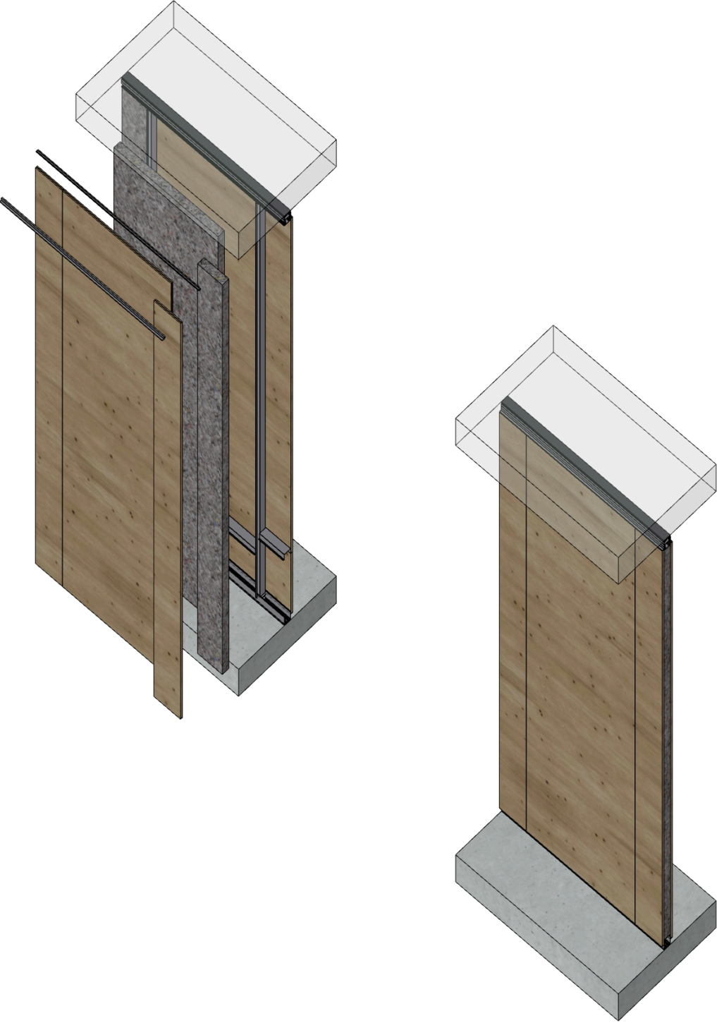
Figure A9. Wall System by VetroIn.
