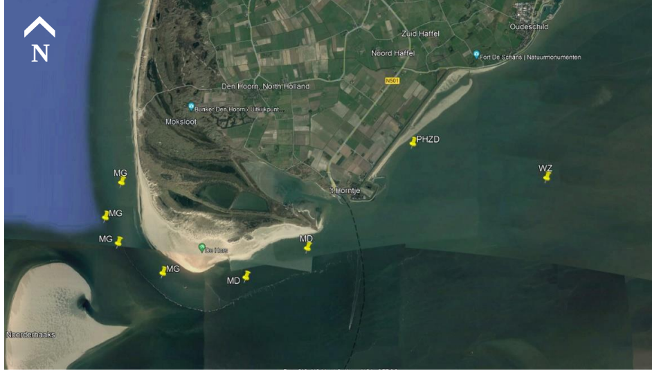
Figure 3. Various locations were sampled around the Dutch barrier island Texel: Molengat (MG) tidal channel, Marsdiep (MD) tidal inlet, near the Prins Hendrikzanddijk (PHZD) coastal nourishment and Waddenzeel (WZ). The North Sea is on the left side of the image, the Waddenzeel back barrier basin on the right side.
