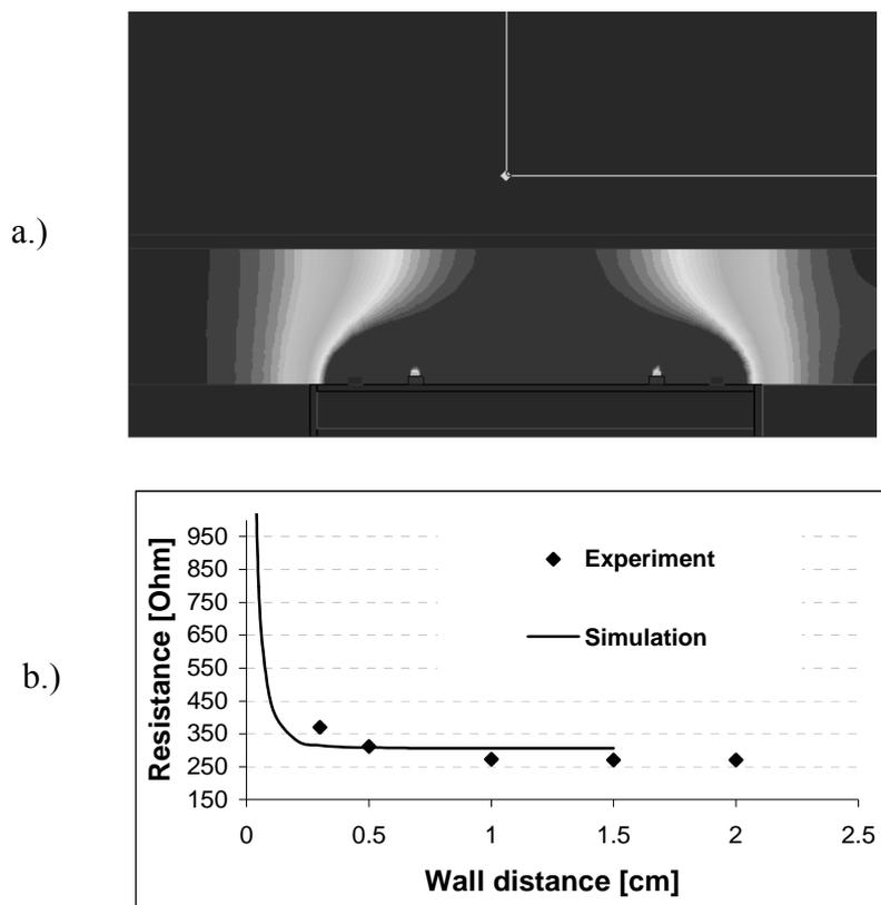
Figure 9. a.) Electrical-field distribution limited by the vessel wall
