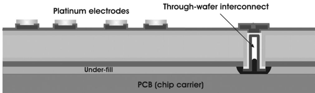
Figure 14. Through-wafer interconnects, with electrodes as the sensor example
