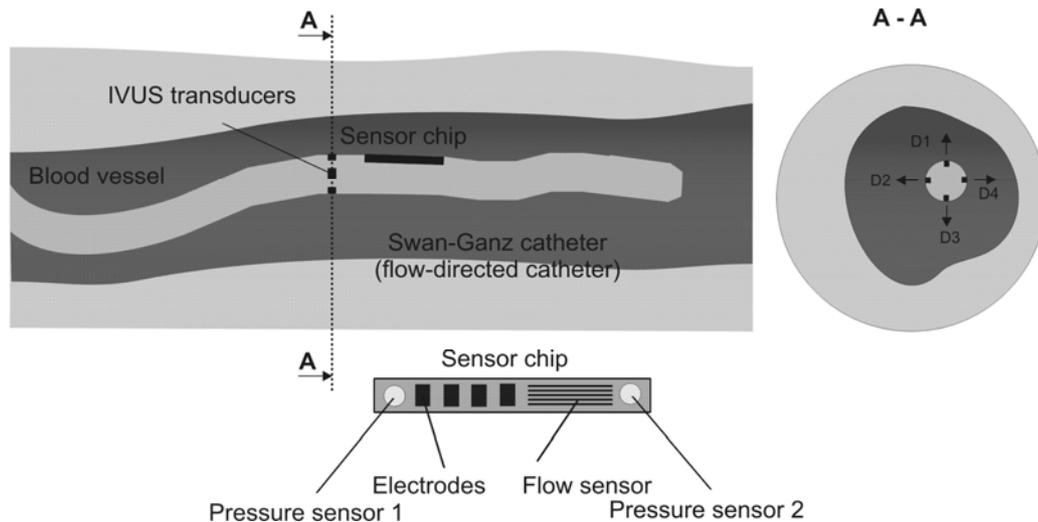
Figure 3. Schematic of the medical probe
