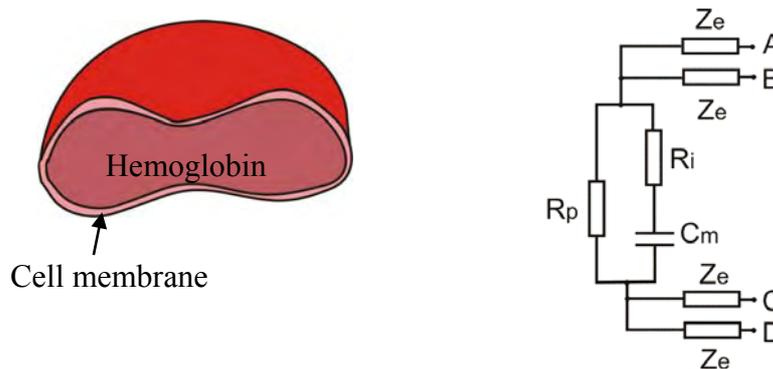
Figure 8. The electrical model of blood ( $R_p$ =plasma resistance,  $R_i$ =internal cell resistance,  $C_m$ =cell membrane capacitance,  $Z_e$ =electrode polarisation impedance)
