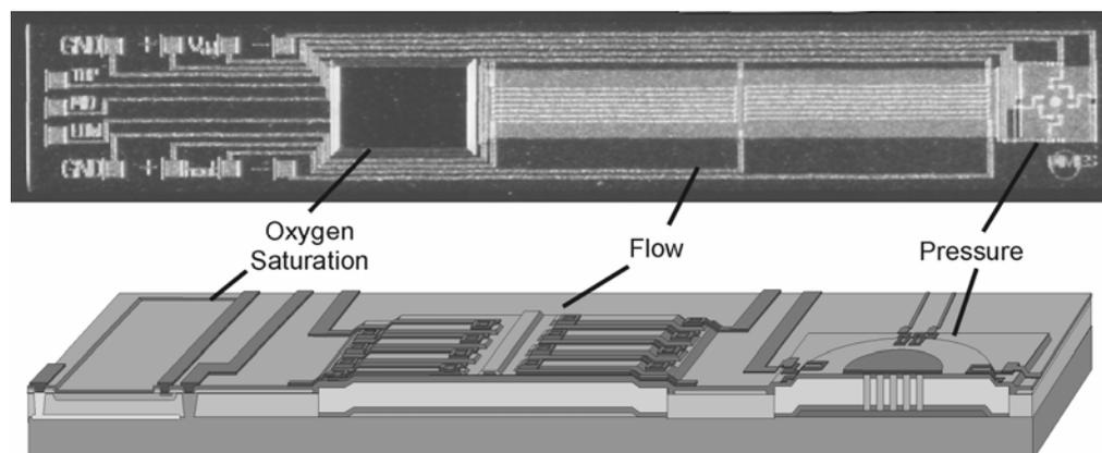
Figure 10. Chip photograph and schematic of the multi-parameter sensor consisting of an oxygen-saturation sensor, a blood-pressure sensor and a flow sensor
