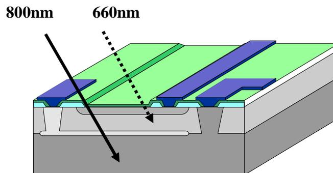
Figure 12. The structure of the oxygen-saturation sensor
