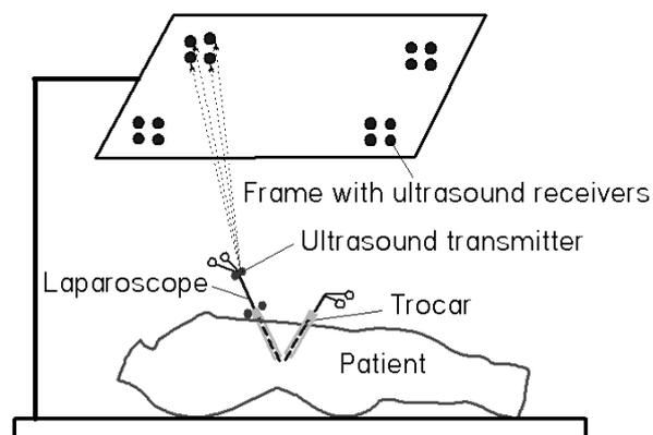
Figure 1. Ultrasound-based system for laparoscopic tools
