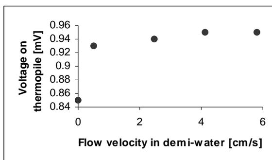
Figure 7. Measurement results when the flow-velocity sensor was tested in demineralised water
