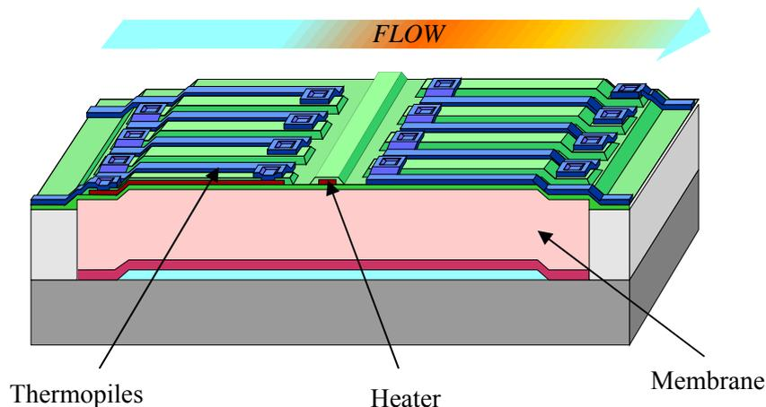
Figure 5. Schematic of the flow-velocity sensor
