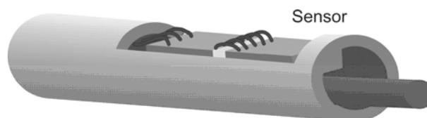
Figure 13. Wire bonding for a catheter sensor
