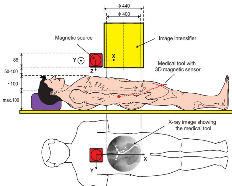
Figure 2. Magnetic-based system for guide wires and/or catheters
