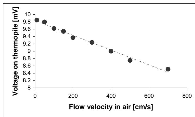
Figure 6. Measurement results when the flow-velocity sensor was in air
