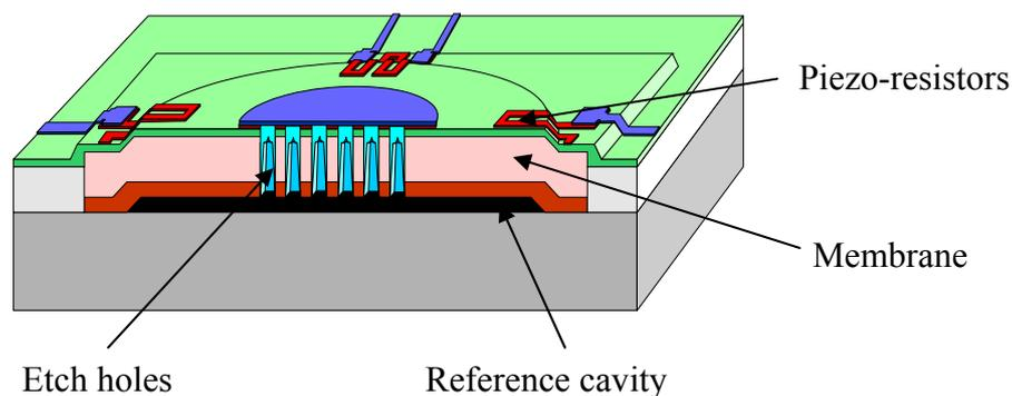
Figure 4. Schematic of the pressure sensor
