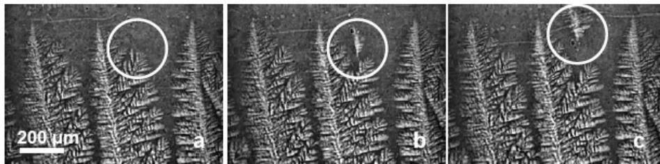
Figure 4.10. In-situ observation of localized fragmentation (in circled region) during the solidification of an Al-20wt % Cu alloy at: (a)  $t=0$  s, (b)  $t=2.25$  s and (c)  $t=4.50$  s.
