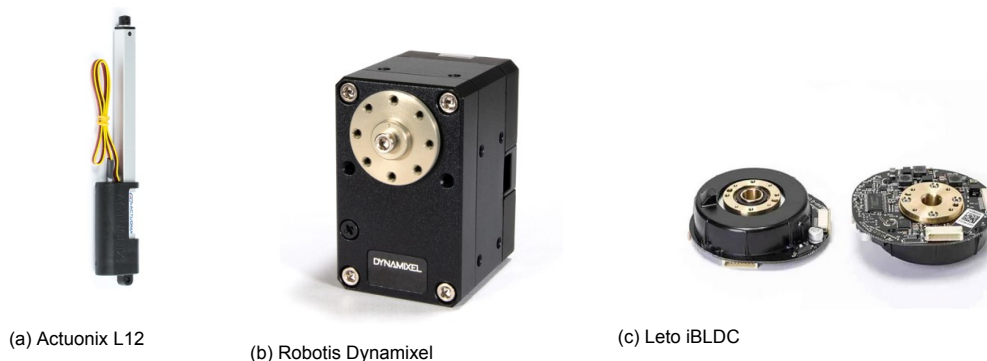
Figure E.5: Suitable servo motor options in three different styles, the linear actuator, the classic servo and the flat pancake model. Selected from the options sourced from rs-online.com , reichelt.com and digikey.nl
