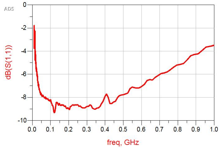
Figure 5.7: Figure shows poor untrimmed S11 of the LNA. This is due to lesser gain of the core LNA than in the simulations.
