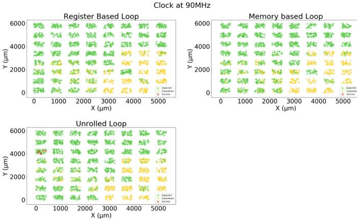
**Fig. 4.** EMFI results of all three tests at 90 MHz (PLL enabled).
