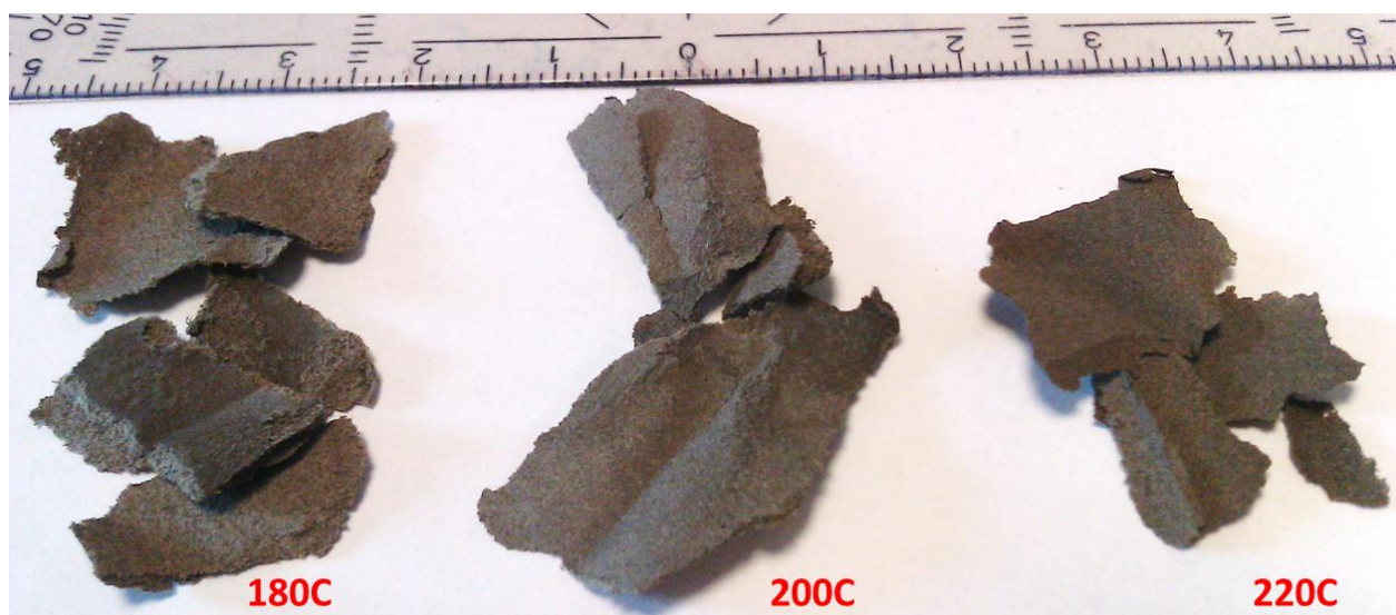
Figure 4-16: WTG after drying
