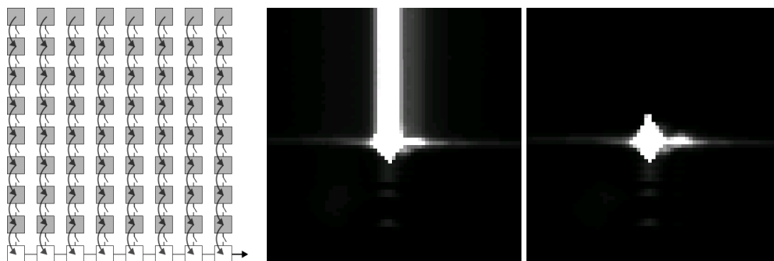
Figure 3.5: Three images illustrating the issue encountered with the spectrometer CCD image. Left displays the readout mechanism of the CCD sensor. Note that the sensor is readout one row at a time, by transferring collected charge via underlying pixels to the output channel on the bottom. The middle and left images compare a CCD image obtained with (right) and without (middle) the use of a shutter. Without a shutter, pixels are continuously exposed, also during readout. The CCD system will misinterpret the output signal resulting in an innacurate image.
