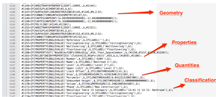
Figure 4.7: STEP Encoding of .ifc file, a # starts every line followed by the entity definition. The = names the entity. The parameters (between brackets) are (among others) empty ($), a number, a list, a string, or the ID of other entities [Arroyo Ogori et al., 2018]. Image taken from https://blog.areo.io/content/images/2016/01/IFC_file_contents-1.png
