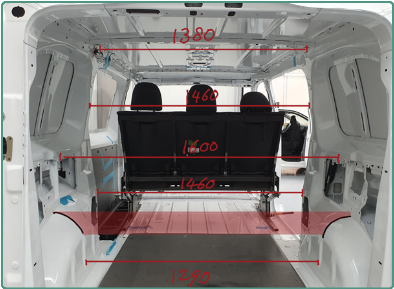
Figure 3.5.2 Width dimensions in the K0 body
