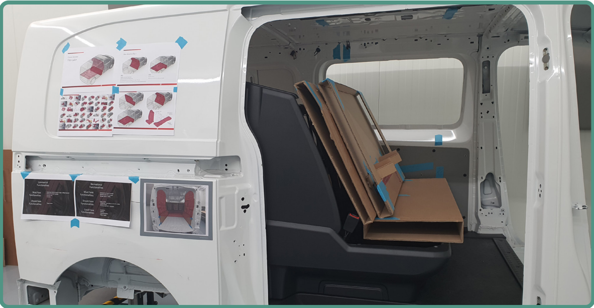
Figure 3.2.5 Increased backrest thickness due to double back
