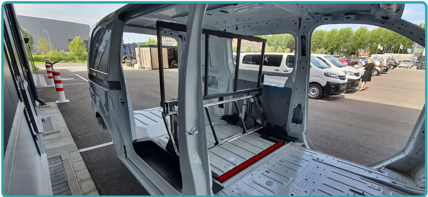
Figure 5.2.2 A crossbar could help distributing the forces applied on the body of the vehicle
