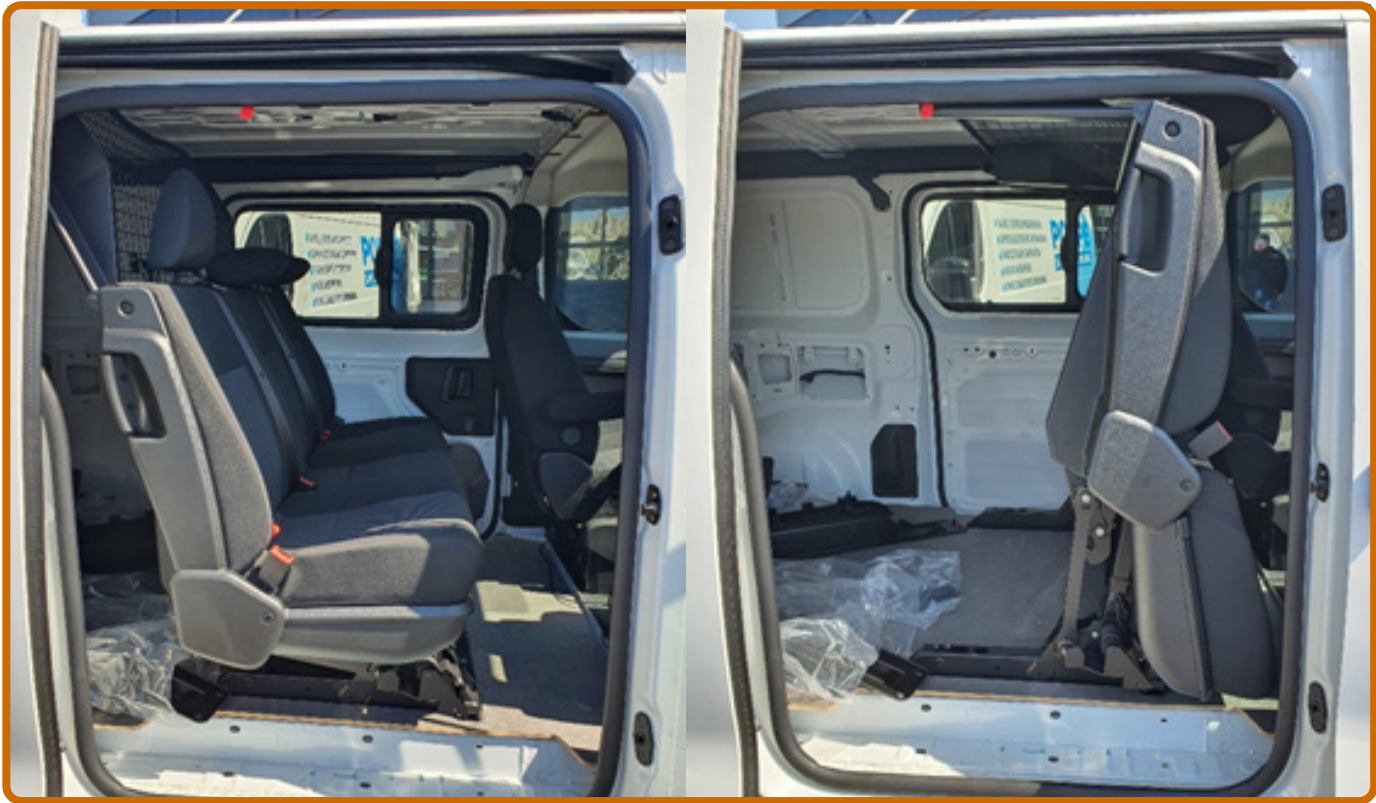
Figure 4.2.2 The additional cargo space that the flex cab enables
