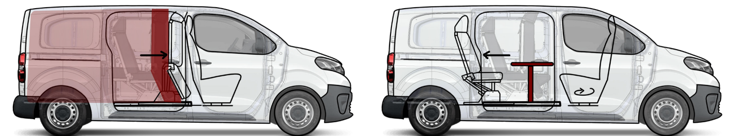
Figure 5.1.1 Sliding rail positions with increased cargo space or living room area
