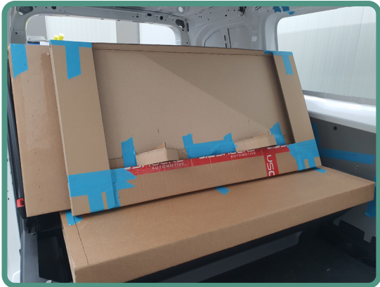
Figure 3.2.3 the backrest with bolsters
