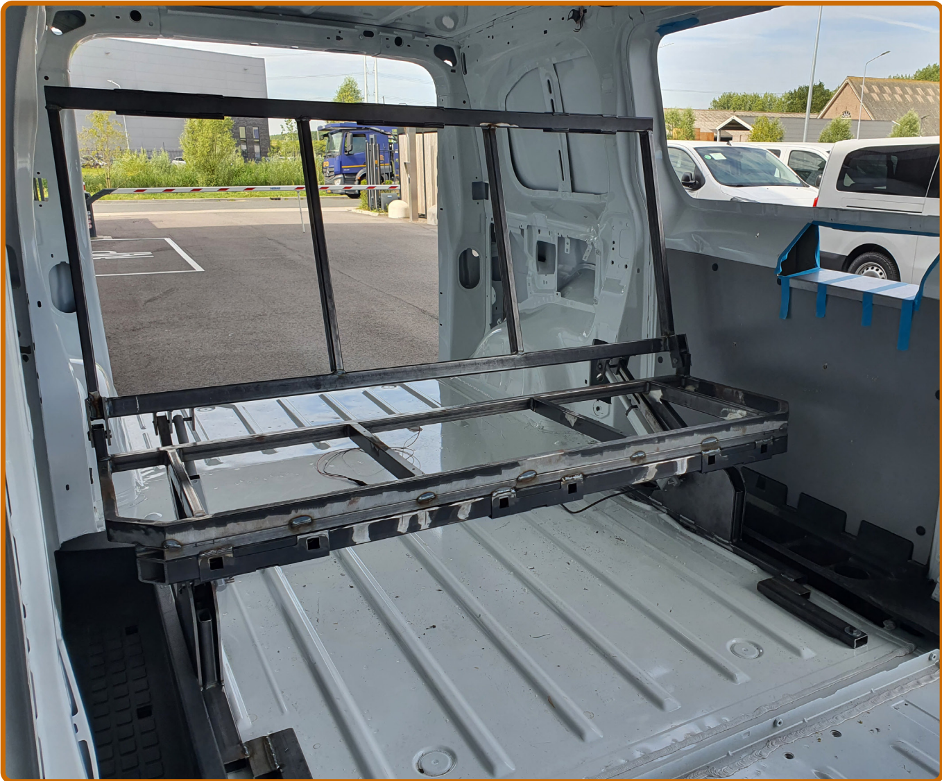
Figure 4.6.4 Mechanical framework in K0 body
