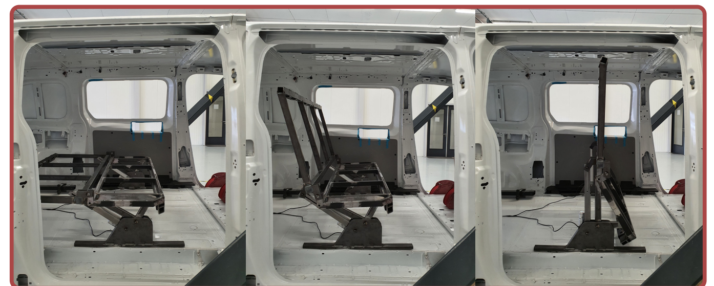
Figure 2. The transitions of the mechanical framework into all three positions
