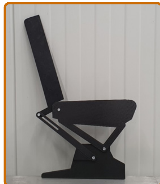
Figure 4.5.1 3D printed mockup to evaluate the rotation points
