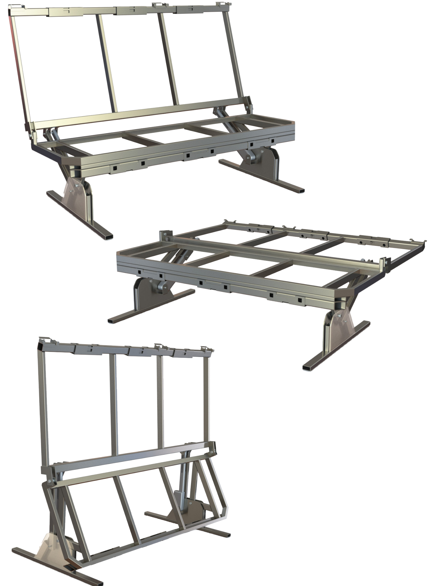
Figure 4.5.2 The CAD framework in seating, sleeping and flexed position
