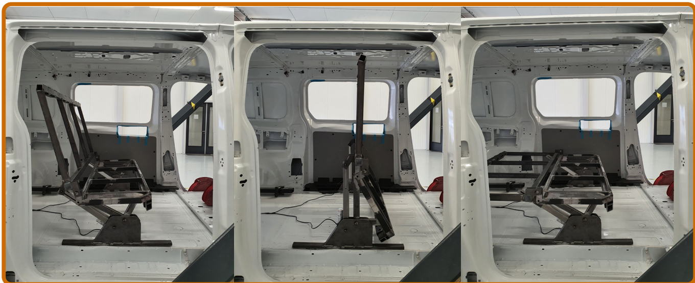
Figure 4.6.2 The transitions of the mechanical framework into all three positions
