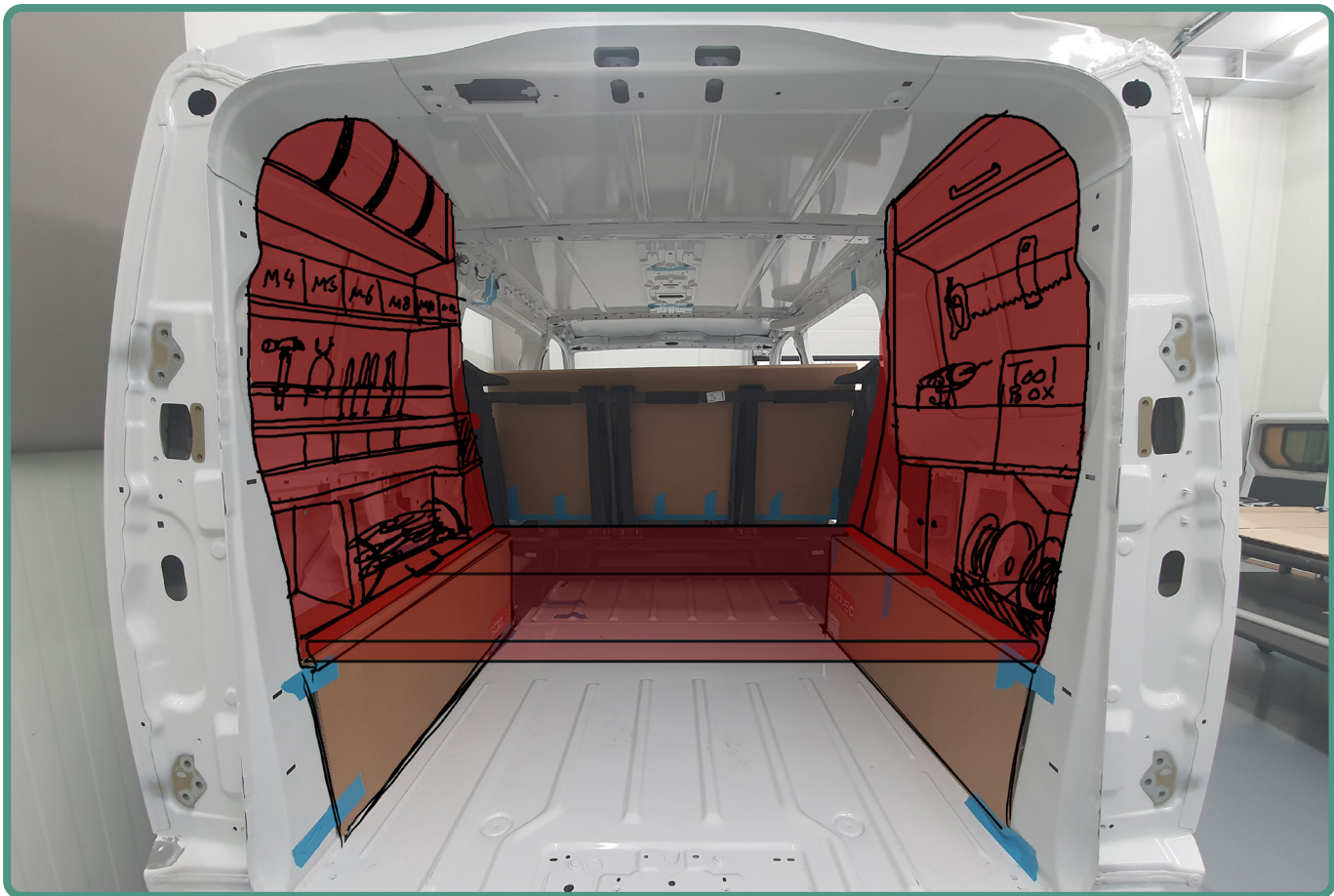
Figure 3.6.3 Possible commercial layout with the supportive structure and shelves
