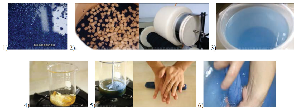
Figure 1. Main steps for Dominique's customized pigment preparation process. (These images were taken from the officially released video of the process. 1) Smashing and washing; 2) Ball mill grinding; 3) Standing and collecting sedimentation; 4) Melting pine resin, mastic and wax; 5) Kneading the paste; 6) Lukewarm lye scrubbing).
