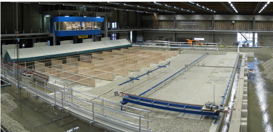
Figure 4.1: Experiment setup in the Delta Basin with at the left side the wooden wave guiding walls and at the bottom the Mobile Measuring Bridge
