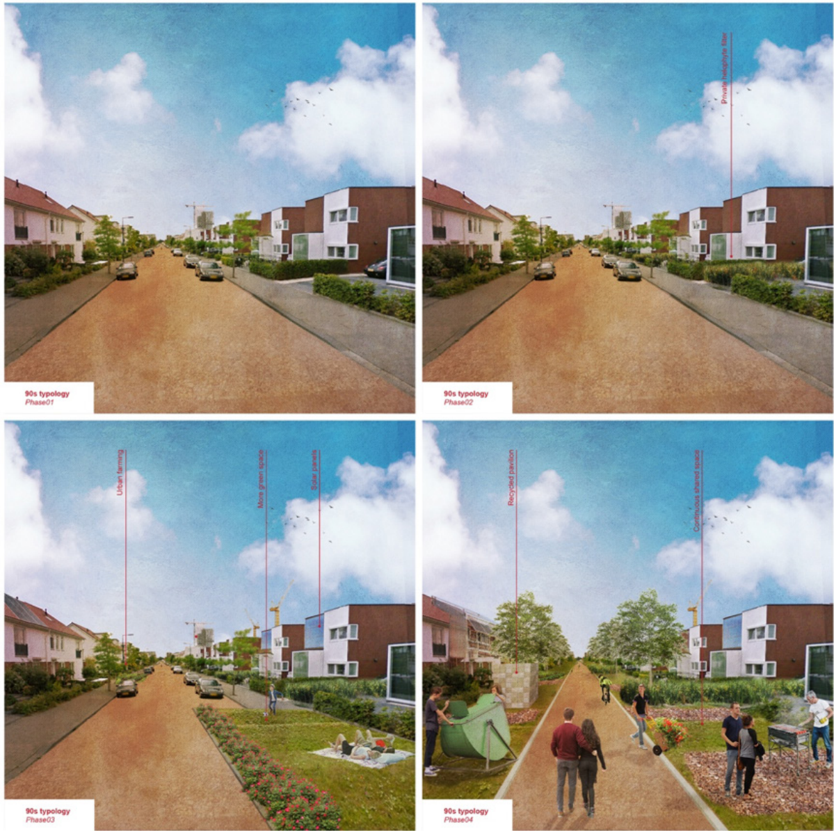
Fig 3.3 The Maya-inspired approach beholds a decentralized services of waste and water to bring the end-user closer to the system. This is done in the large open areas for water and greenery and supplement the advantages of the present designs - including good energy efficiency of housing, a separated sewer system, high rainwater infiltration, and natural methods for cleaning open water - whilst turning fertile soil into a public asset that reorganises water flows and waste processing on a communal scale.
