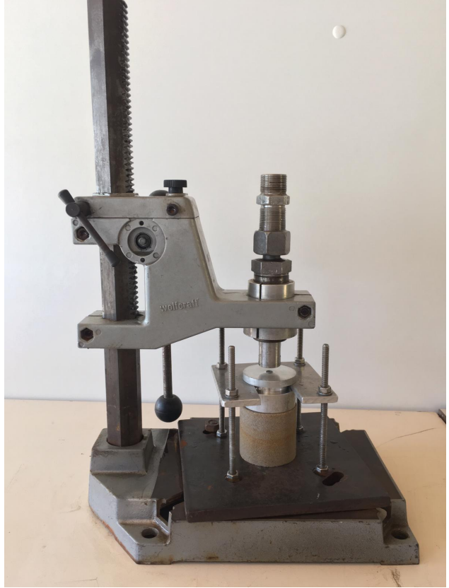
(b) Photo of the setup. A rock sample is compressed with an aluminium adapter on top (experiment (C)).
