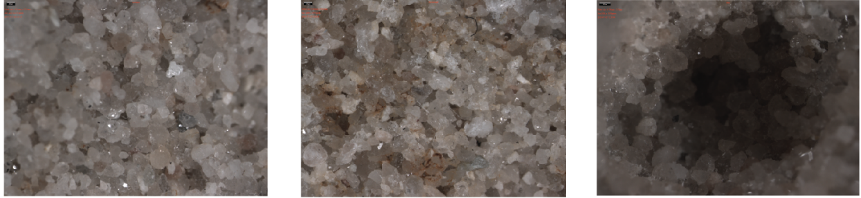
Figure 4.23: Microscopic images of Bad Durkheim samples. From left to right: sample with cavitation erosion, undamaged sample and a sample with a jetted hole. Not much difference is visible.
