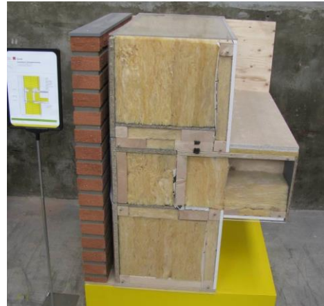
Figure 3-5 Insulation according Passive-House standard \pm 0.35 m and R_c 9,8 Km^2/W (Van den Ham, 2012)
