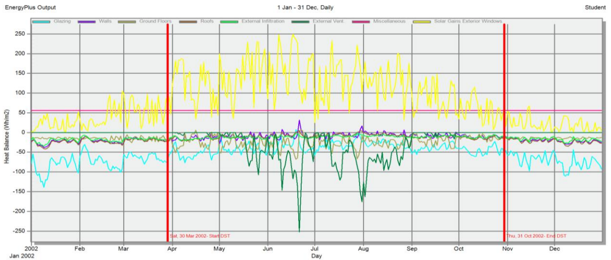
Figure 13-4 Daily heat losses and gains of the dwelling subdivided in different components
