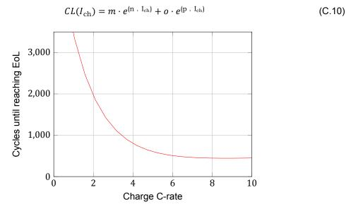
Figure C.4: Effect of charge C-rate on cycle life according to model Omar et al.[44]
