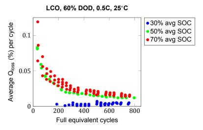
Figure 3.13: Effect of average SOC on cycle aging LCO
