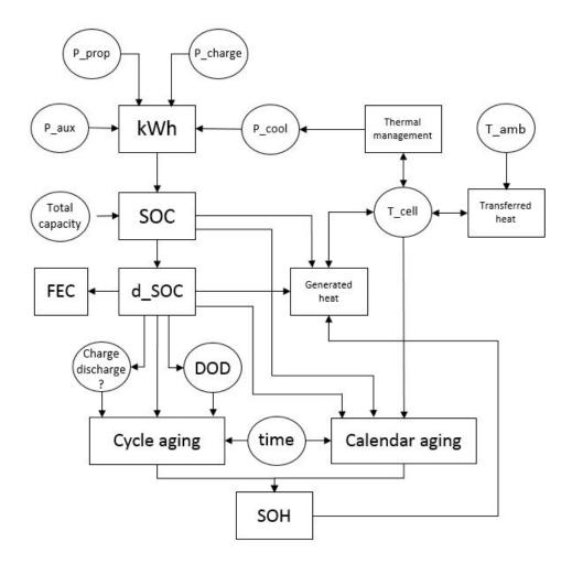
Figure 4.5: Schematic representation of calculation steps in Simulink
