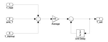
Figure D.9: Subsystem thermal model/battery
