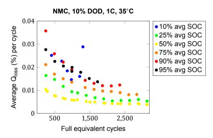
Figure 3.14: Effect of average SOC on cycle aging NMC
