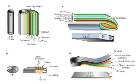
Figure 2.2: Different types of cell design, cylindrical (a), coin (b), prismatic (c) and pouch (d) [57]
