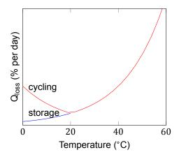
Figure 4.1: Effect of temperature on aging rate
