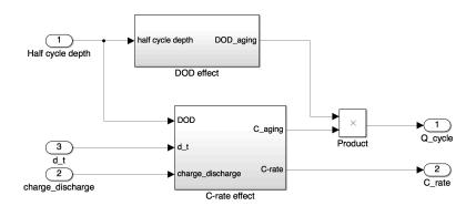
Figure D.18: Subsystem cycle aging
