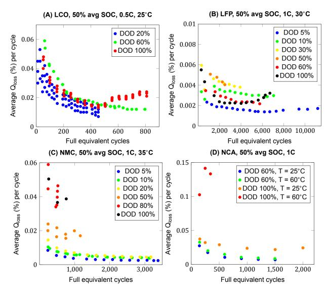
Figure 3.11: Effect of depth of discharge (DOD) on cycle aging
