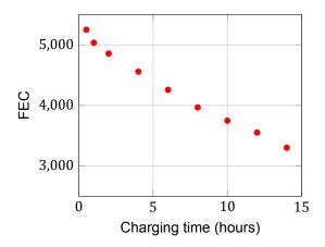
Figure 5.7: Simulation results for cycling at 50% DOD and variable overnight charge strategy
