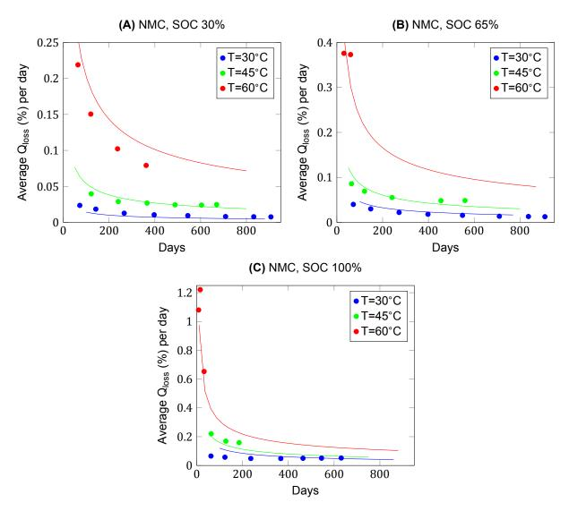
Figure 4.10:  $\alpha$  = 0.06,  $\beta$  = 1.092,  $\kappa_1$  = 0.0001,  $\kappa_2$  = 0.0211, NMC 5.3 Ah cell from SIMCAL aging tests [15]
