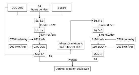
Figure 5.23: Steps to determine optimal battery size for 5 year battery life ferry
