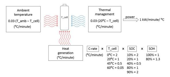
Figure 4.6: Schematic representation of thermal part in proposed aging model
