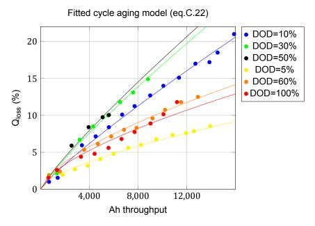
Figure C.8: Cycle aging data fitting (10% ≤DOD ≤50%)
