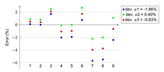
Figure E.14: Distribution of the errors of the simulation compared to Keil data[32]
