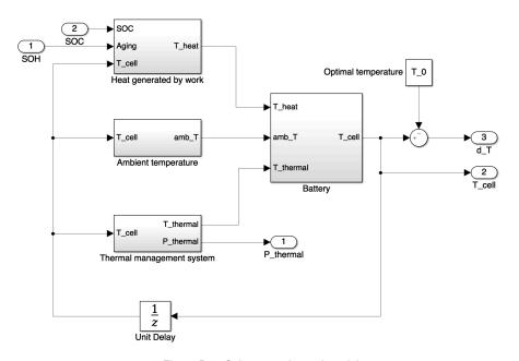
Figure D.5: Subsystem thermal model
