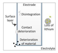
Figure 3.2: Battery half cell representing the five main aging mechanisms
