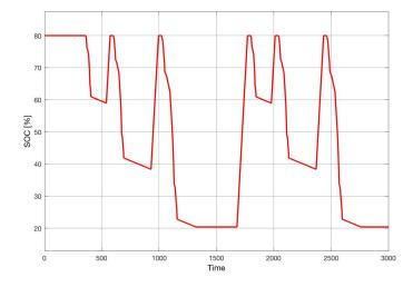
Figure 5.12: State of charge of the 4.5 MWh battery during operational profile 1
