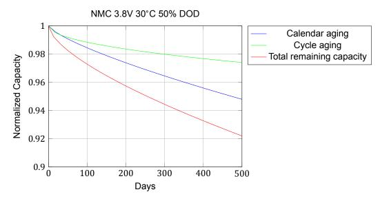
Figure C.6: Remaining capacity according to model by Schmalstieg et al.[55]
