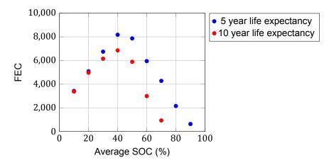
Figure 5.4: Simulation results for cycling at 20% DOD and 1C with different average SOC
