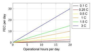
Figure 5.20: Estimation of performed FEC per day based on C-rate and operational hours per day
