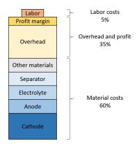
Figure 2.3: Cost components for lithium-ion battery cells [49]
