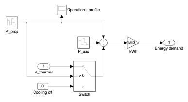
Figure D.3: Subsystem operational profile/ship
