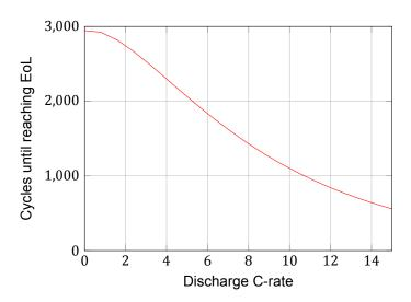
Figure C.2: Effect of discharge C-rate on cycle life according to model Omar et al.[44]
