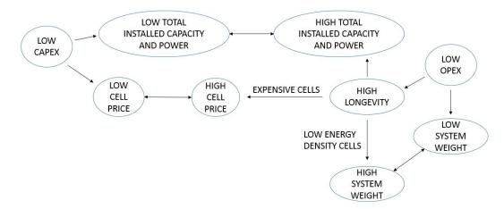
Figure 2.6: Selecting a battery cell on CAPEX and OPEX
