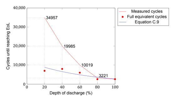
Figure C.3: Effect of depth of discharge on cycle life according to model Omar et al.[44]
