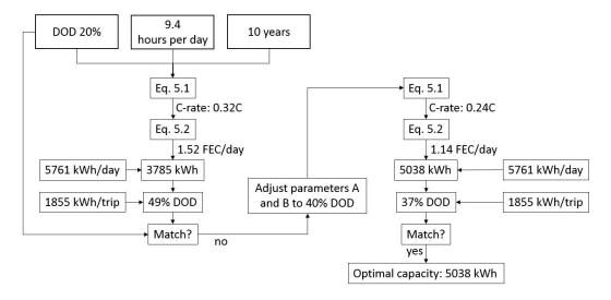
Figure 5.22: Steps to determine optimal battery size for 10 year battery life tug
