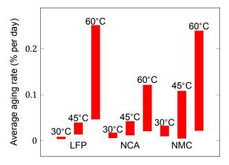
Figure 3.4: Minimum and maximum aging rate at 30% SOC
