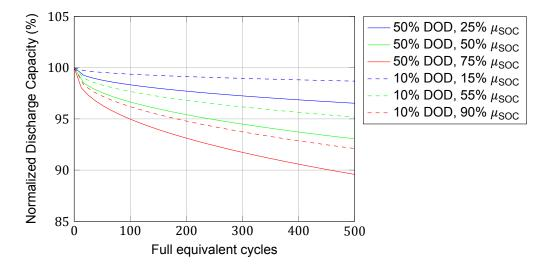
Figure C.5: Effect of DOD and mean SOC on cycle life according to model Saxena et al.[54]
