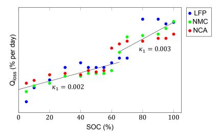
Figure 4.2: Effect of the state of charge on aging rate
