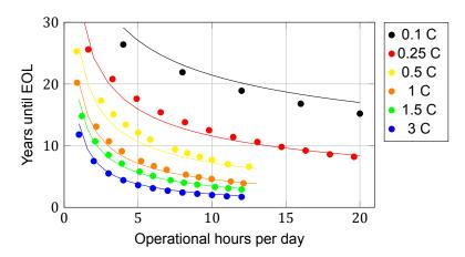
Figure 5.19: Years until EOL per C-rate and operational hours per day at 20% DOD
