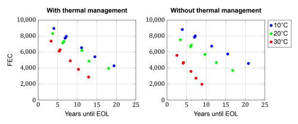
Figure 5.8: FEC and years until EOL at different ambient temperatures with thermal management system
