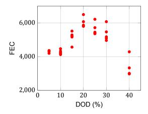
Figure 5.3: Performed FEC at EOL after 10 years for different DOD at different C-rates
