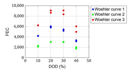
Figure 5.6: Performed FEC at EOL after 10 years with different Woehler curves
