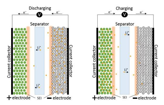
Figure 3.1: Schematic representation of a lithium-ion battery
