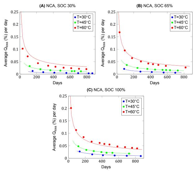
Figure 4.9:  $\alpha$  = 0.077,  $\beta$  = 1.063,  $\kappa_1$  = 0.002,  $\kappa_2$  = 0.003, NCA 7 Ah cell from SIMCAL aging tests [15]
