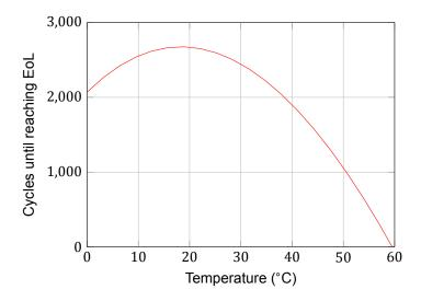
Figure C.1: Effect of temperature on cycle life according to model Omar et al.[44]
