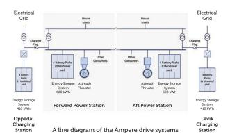
Figure A.2: Line diagram of Ampere drive systems[20]
