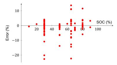
Figure 4.14: Distribution of the absolute simulation errors at different SOC levels
