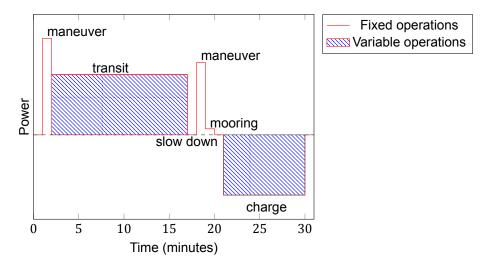
Figure 5.15: Typical profile for a single job of a ferry
