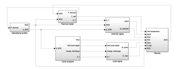
Figure D.1: Main screen of the aging model
