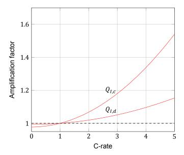
Figure 4.4: Effect of C-rate on cycle aging rate
