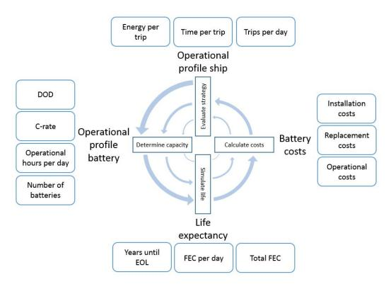
Figure 5.9: The four steps for battery optimization
