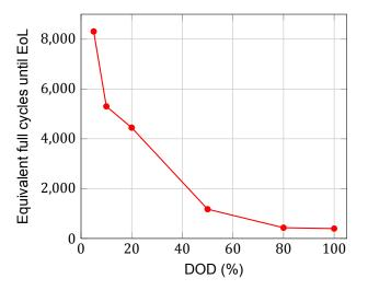
Figure 4.3: Woehler curve of aging data for NMC battery from figure D.19 (C)
