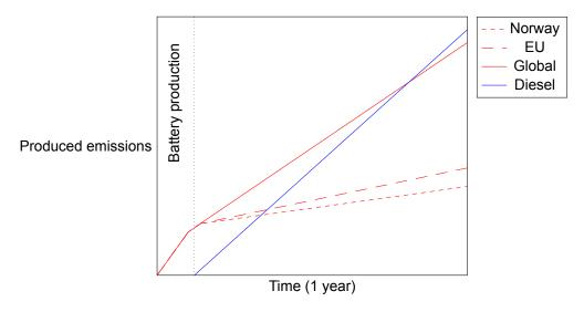
Figure A.5: Payback time on emissions fully electric vs. diesel
