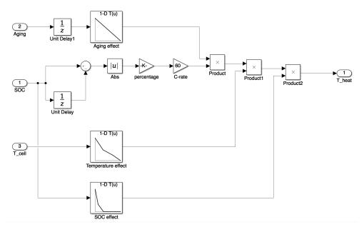
Figure D.6: Subsystem thermal model/heat generation
