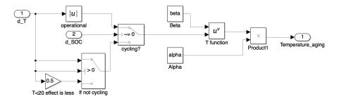
Figure D.16: Subsystem calendar aging/temperature aging
