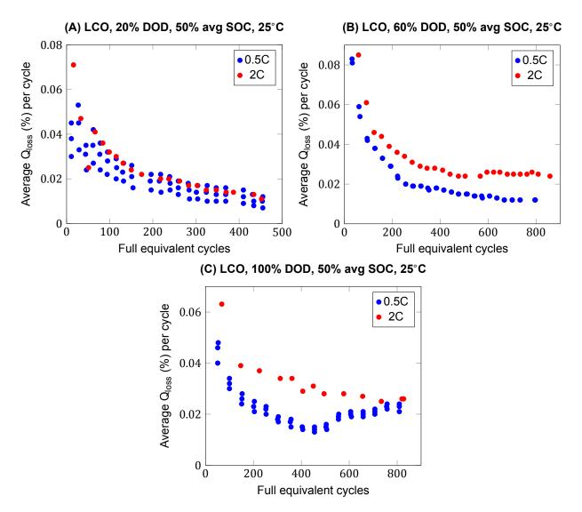
Figure 3.12: Effect of C-rate on cycle aging rate for LCO
