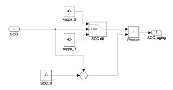
Figure D.15: Subsystem calendar aging/SOC effect
