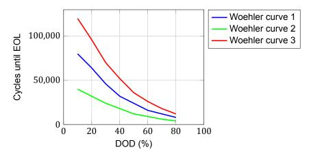
Figure 5.5: Three different Woehler curves to represent three batteries with different aging characteristics
