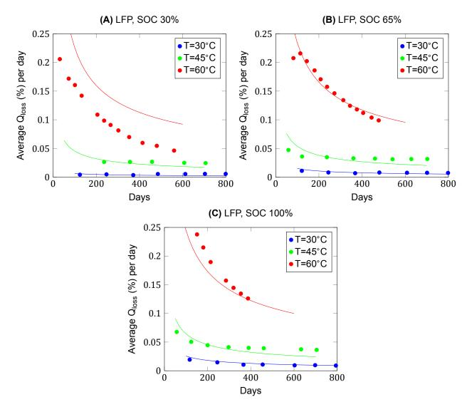
Figure 4.8:  $\alpha$  = 0.038,  $\beta$  = 1.108,  $\kappa_1$  = 0.002,  $\kappa_2$  = 0.003, LFP 15 Ah cell from SIMCAL aging tests [15]
