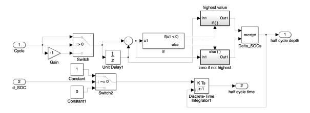
Figure D.13: Subsystem cycle analysis/Calculate half cycle depth and time
