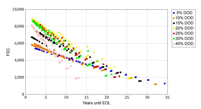
Figure 5.1: Results of general analysis simulations for performed FEC and years until EOL
