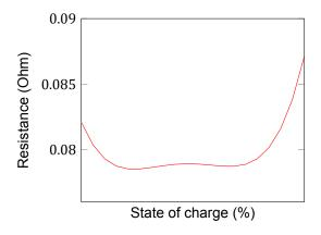
Figure 3.3: Example of a resistance curve of a lithium-ion battery[31]
