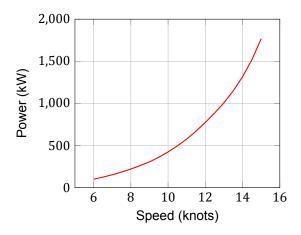
Figure F.1: Vessel speed and required power for DRPa9919 ferry
