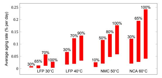
Figure 3.7: Minimum and maximum aging rate compared for variable SOC
