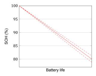
Figure 4.7: Average variation of 6% in aging for similar cell type under similar testing conditions
