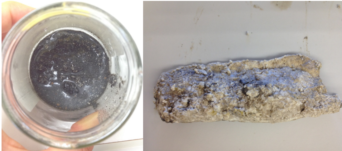
Figure 20 - FOG deposit samples collected from kitchen drains (left) and lateral house connections (right), showing their appearance, shape and color.
