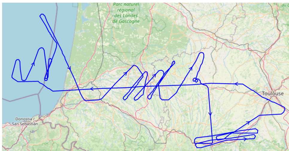
Figure 8.1: Lagrangian pattern flown during a SENS4ICE research flight. On the day of the flight, a warm front moved from the Atlantic coast toward Toulouse. The flight pattern was chosen such that it approximately matched the speed of the warm front. The blue arrows indicate the flight direction of the aircraft. Map from OpenStreetMap .
