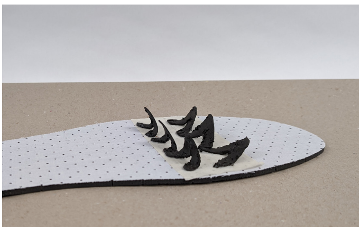
Figure 78. Haptic feet spikes demonstrator in its resting position (Top) and progressively actuated positions (Left-Right)
