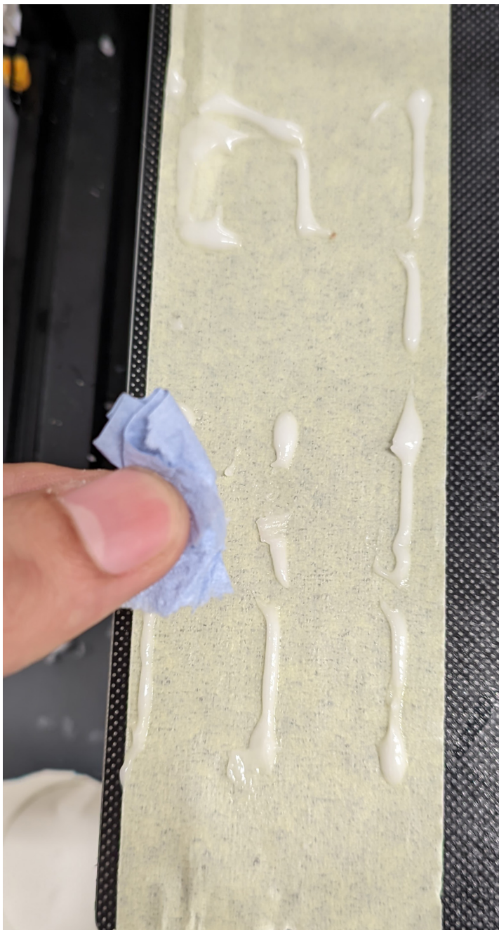
Figure 52. Third attempt with baking soda analogue resulted in improper flow along with significant step skipping, material did not cure (lack of either part A or part B)
