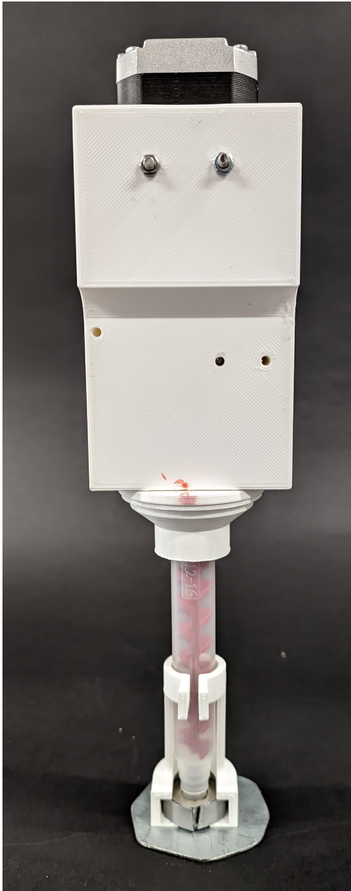
Figure 29. Complete mixing nozzle and stirrer assembly with attached permanent magnet
