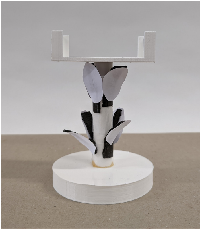
Figure 77. (Top) Pine cone demonstrator at resting position (Top right) Demonstrator when magnet attracts the free tips of the magnetized segments. (Right) Demonstrator when free tips repel the magnet
