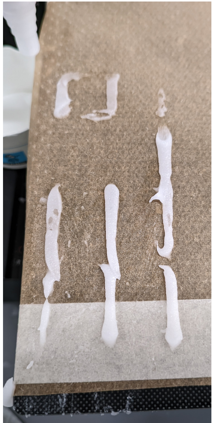
Figure 51. Final result of the test samples G-code, towards the end flow rate significantly dropped
