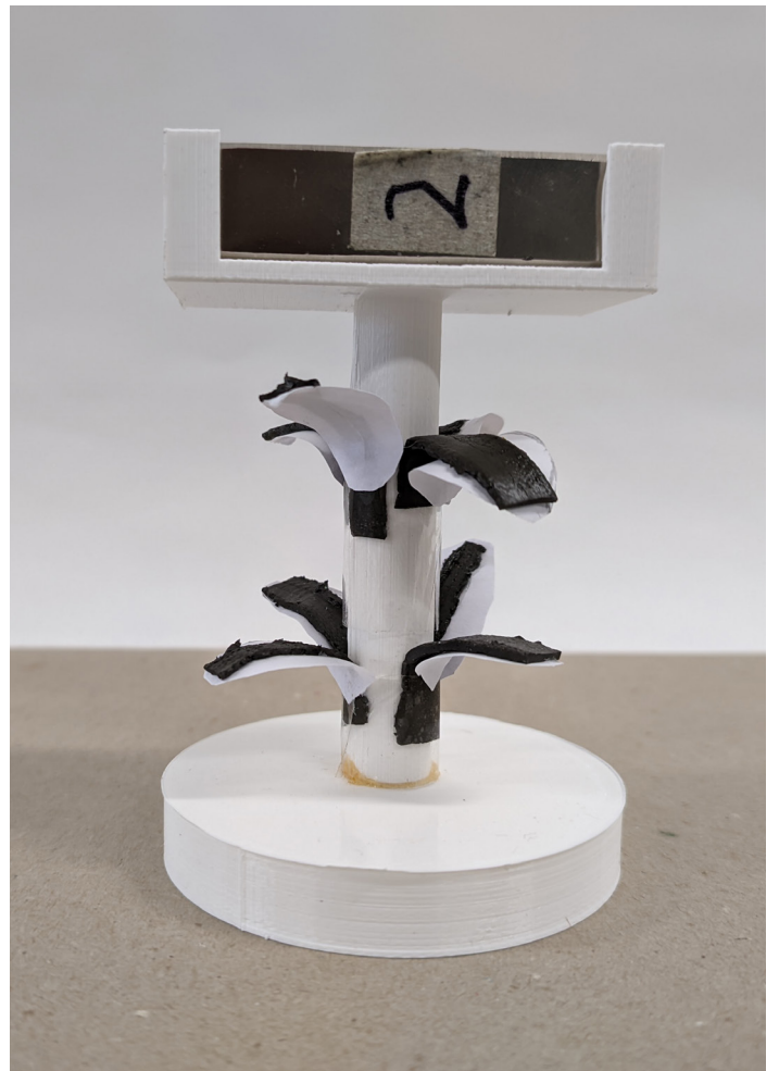
Figure 77. (Top) Pine cone demonstrator at resting position (Top right) Demonstrator when magnet attracts the free tips of the magnetized segments. (Right) Demonstrator when free tips repel the magnet
