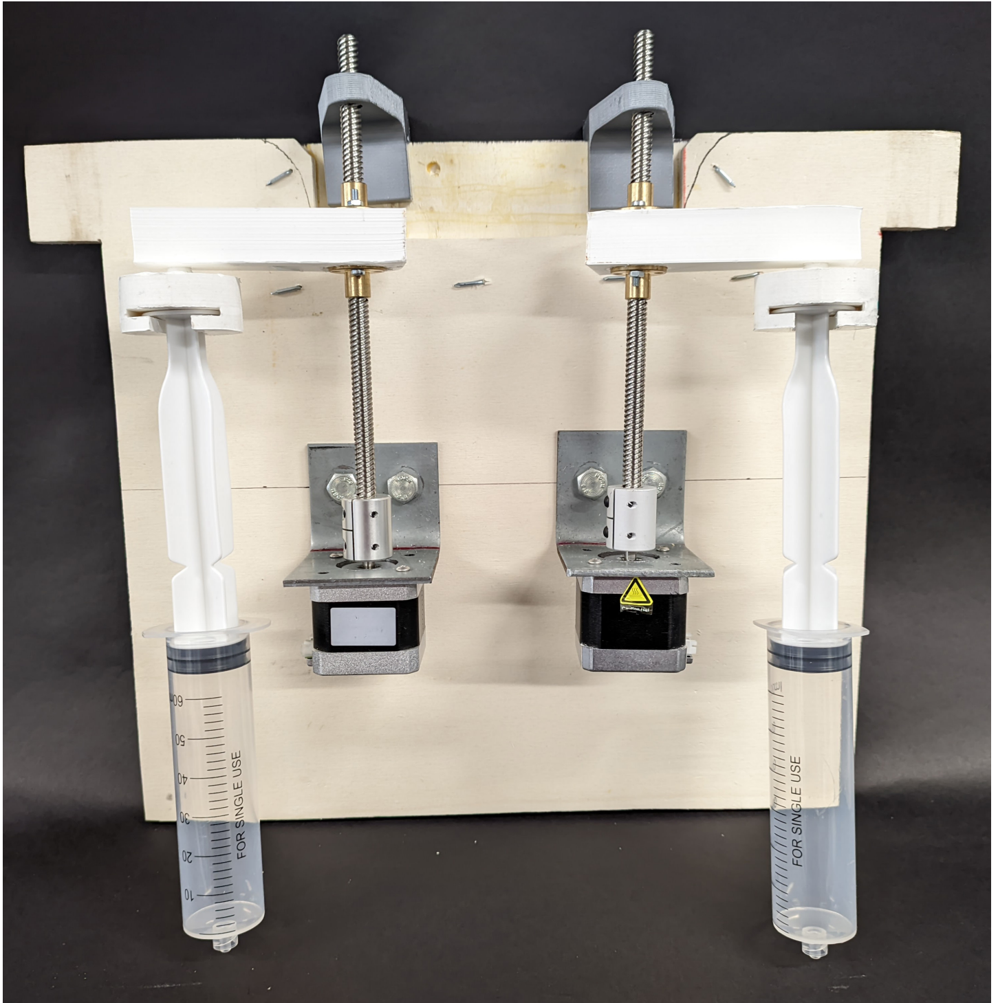
Figure 33. Entire piston extrusion assembly, including motors, lead screws, lead screw nut+connector block, lead screw supports, piston connectors and syringes
