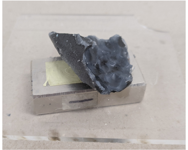
Figure 80. (Left) Pipe valve demonstrator coated in resin (Bottom left) Demonstrator when there is a magnet placed on its right (unseen). (top) Demonstrator between two attracting magnets, showing anomolous shape change. (Above) irregular deformation seen with magnet placed below the demonstrator
