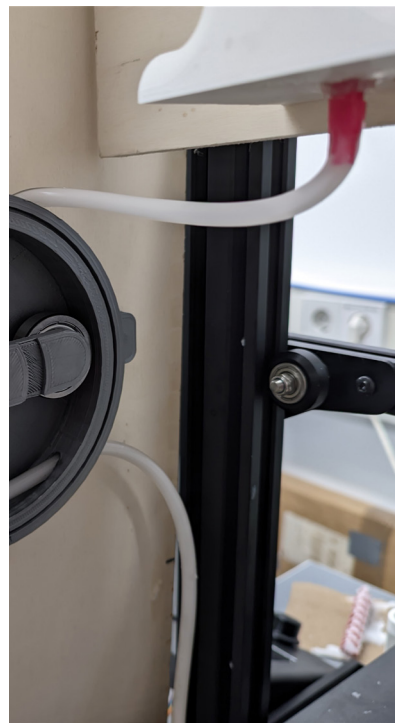
Figure 36. Luer lock attachment in place and its connection to the peristaltic pump
