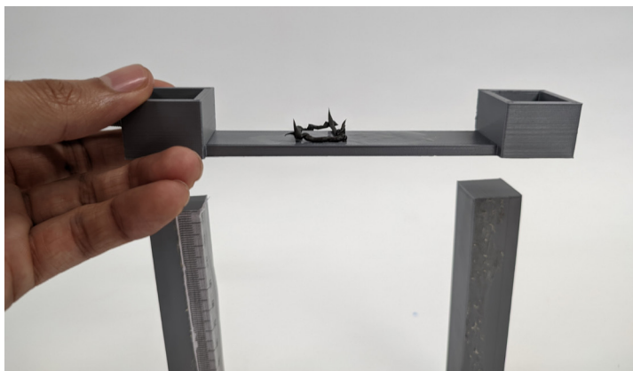
Figure 72. Material shows complete immediate shape recovery upon removal of magnetic field
