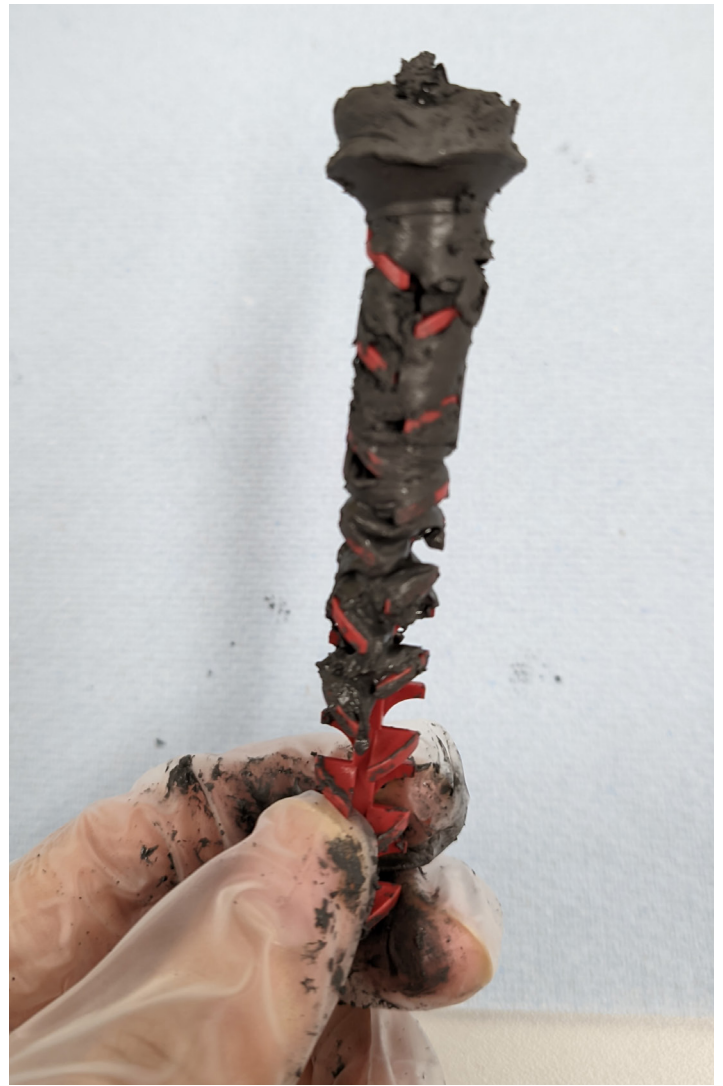
Figure 46. Material curing before it was able to reach the bottom of the entire extruder during testing the piston extrusion system
