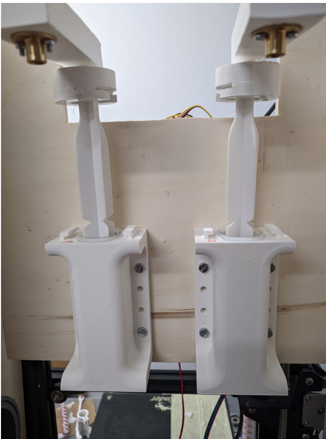
Figure 35. syringe holders with syringes, piston connectors and connectorion blocks
