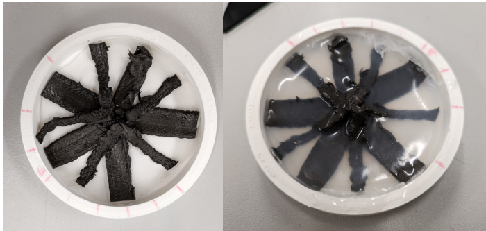
Figure 79. Suction Demonstrator being cast in resin (Top). (Right) progressive steps to actuate the demonstrator
