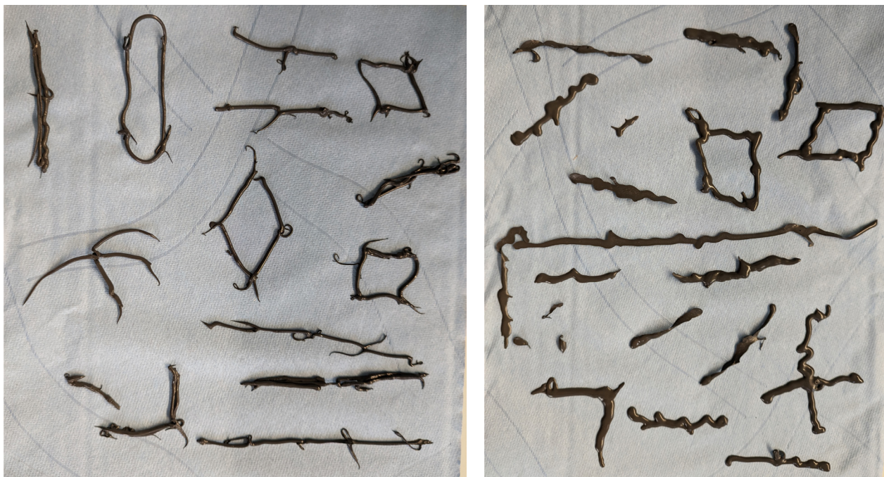
Figure 56. Results of (70-30) (left) and (30-70) mixing ratios of Parts A and B resins
