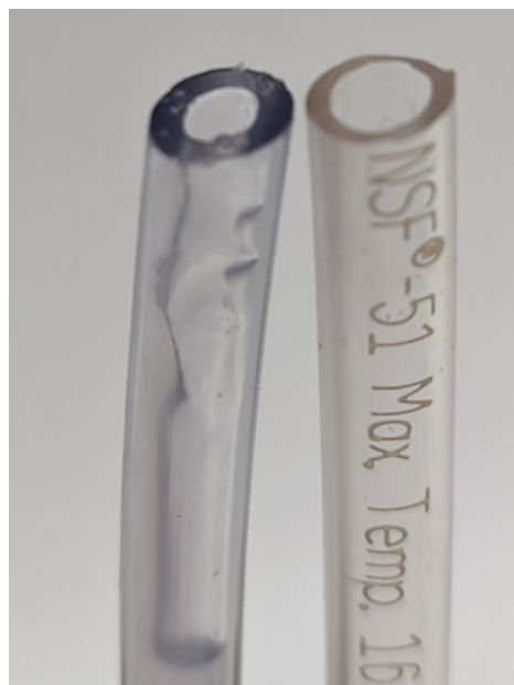
Figure 37. (left) old tube with inner diameter 3mm, (right) new tube with inner diameter 4mm
