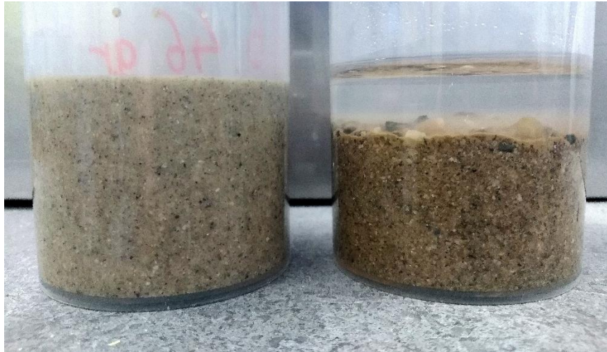
Figure 8.4: Equal amounts of sand (100 gr of soil C) mixed with bentonite (left) and water (right).
