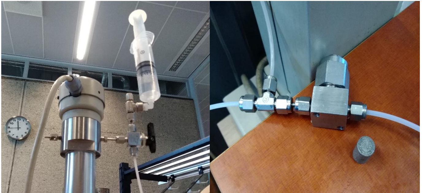
Figure 9.5: Schematization of pressurized foam apparatus. The surfactant solution (contained in the syringe on the left) is pushed by pressurized air through the porous stone (enclosed in the metal housing on the right).
