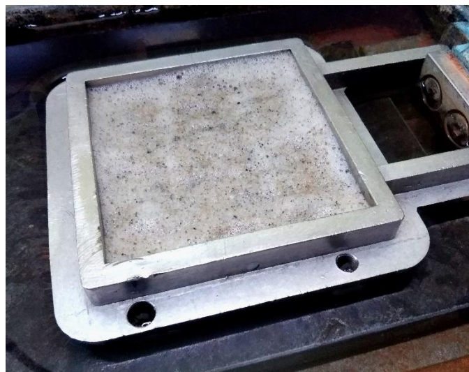
Figure 6.15: Foam-conditioned sample of soil C; prior to fitting porous stone and loading cap.
