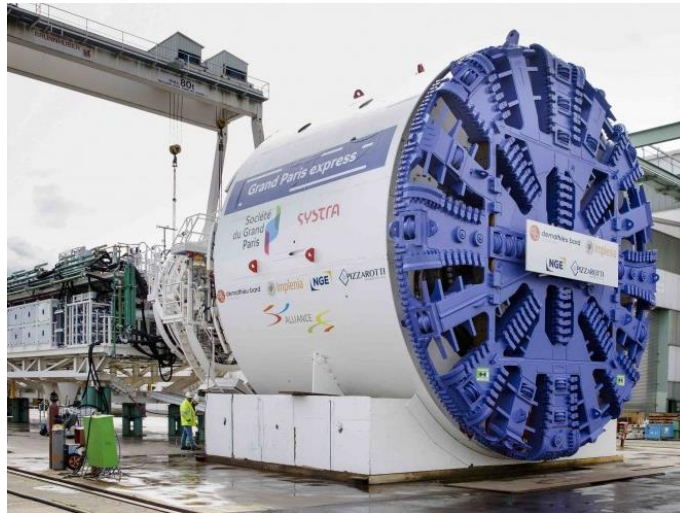
Figure 1.2: TBM cutterhead (in blue) and shield (in white) assembled prior to excavation ( tunnellingjournal.com ).
