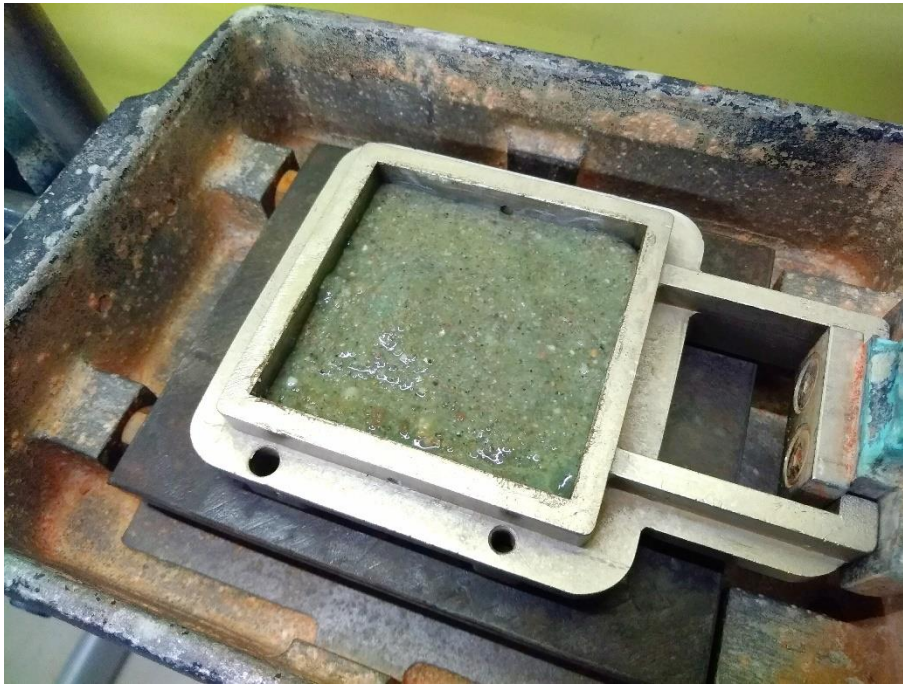
Figure 6.13: Bentonite-conditioned sample of soil C, prior to fitting porous stone and loading cap.
