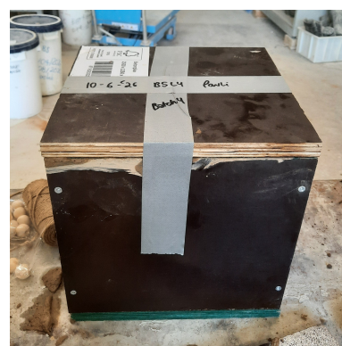
(c) Top plate secured with adhesive tape
