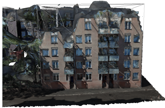
Figure 4.41: Roof of the building B_9 of the MVSM model and the LOD1 CityGML model (transparent box).
