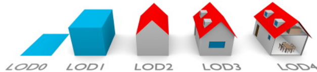
Figure 2.2: The five LODs defined by CityGML (Figure from Biljecki et al. (2016)).
