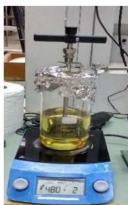
Figure A-1: Test setup for Measuring moisture in oil
