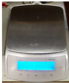
Figure 3-12: Weighing scale used to measure moisture ingress
