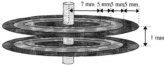
Fig. 5. Experimental version of the circular cross-capacitor.
