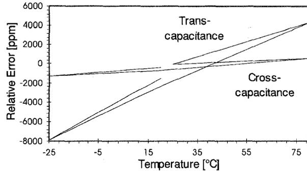
Fig. 6. Capacitance error versus temperature.
