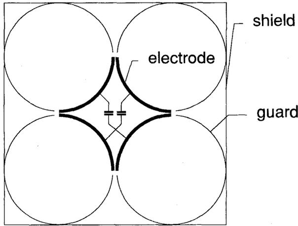
Fig. 2. Cross section of Thompson-Lampard capacitor.
