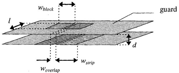
Fig. 4. Strip-block capacitor.
