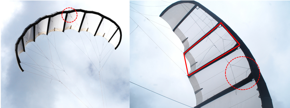
Figure 5.3: Two images of the V3.A kite, where the red quadrilateral indicates one of the spanwise segments and the red dotted circles indicate the bridle fan [60]. The curved lines of the membrane canopy TE in between the strut tips demonstrate the ballooning.
