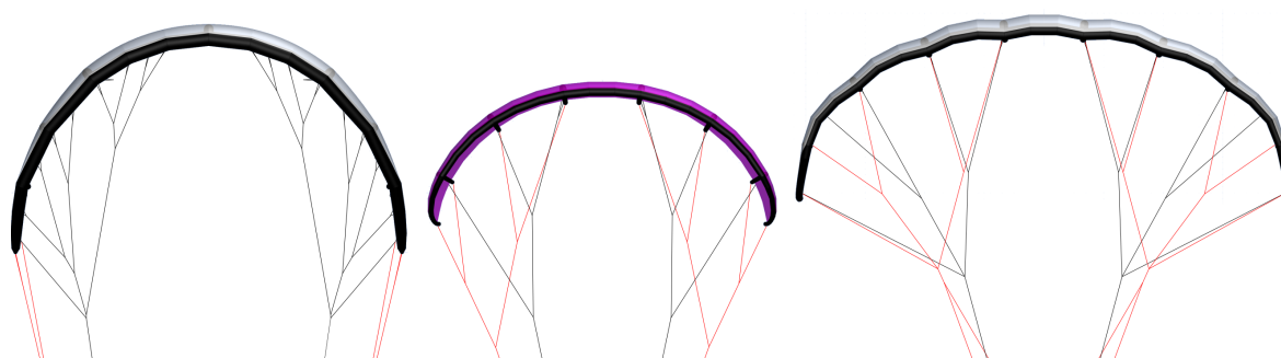
Figure 5.1: Kitepower B.V.'s kite evolution from left to right one sees the: V2, the Hydra and the V3 [60].
