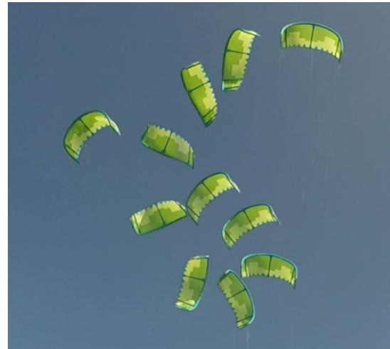
Figure 1.7: Deformation of a LEI surf-kite during a left-turning maneuver [17].
