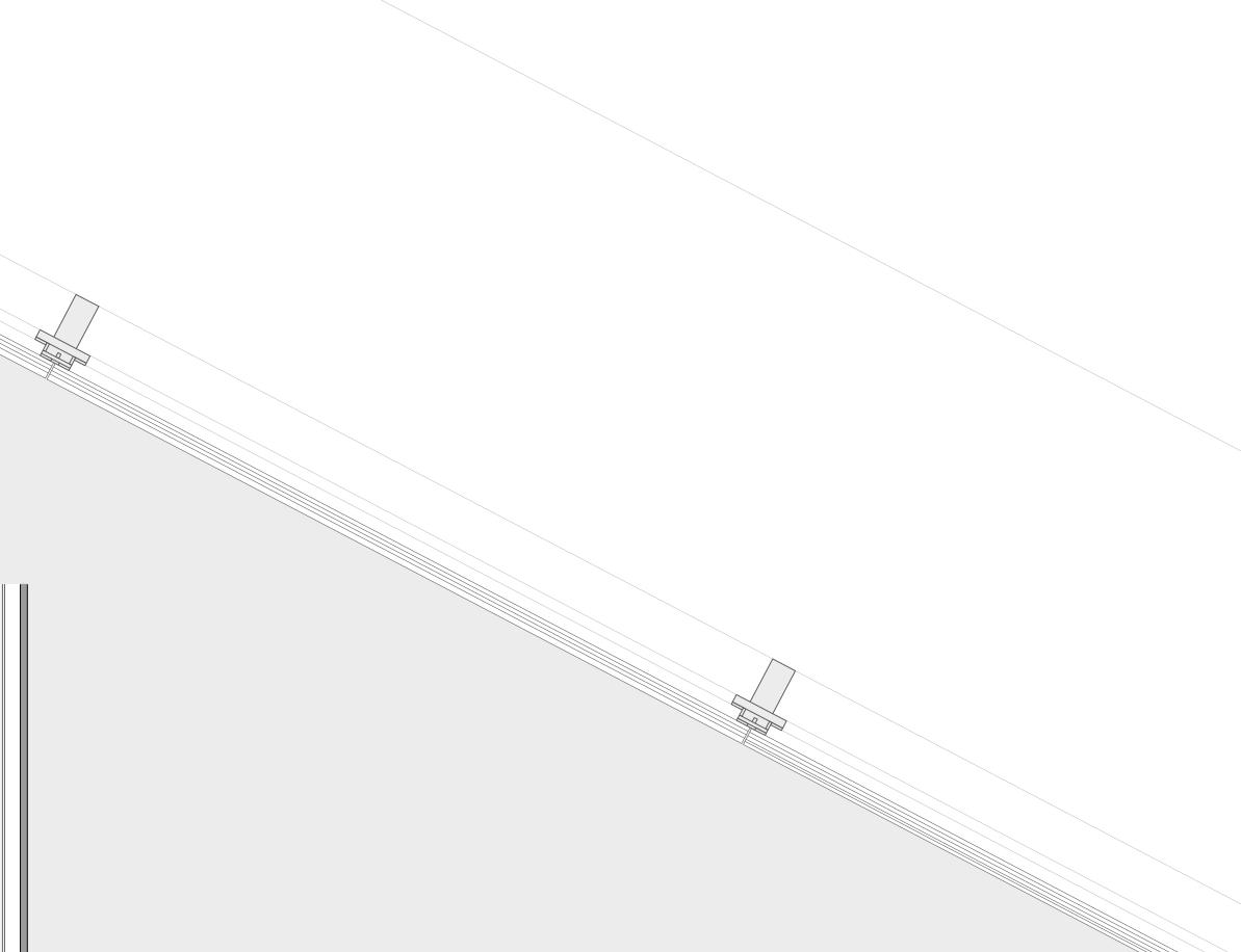
— 1200x3000 mm TAKTL Concrete tile th. 12.7mm, rough II finish — 100x300 mm Steel Frame
