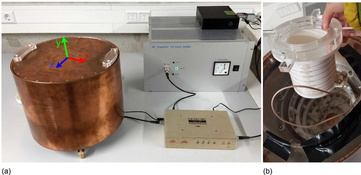
Figure 4.1: a) Prototype of the rotating MRI machine. b) Phantom holder of the Rotating MRI.
