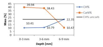
Figure 2: Portlandite and carbonate contents at different depths from exposed surface after 22 days.
