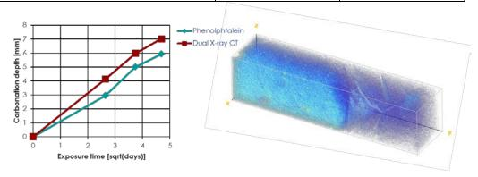
Figure 1: Carbonation depth as measured from dual CT in comparison to phenolftalein indicator.
