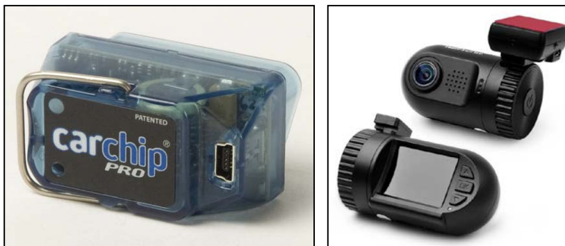
Figure 15 - FOT Equipment: CarChip Pro OBD2 Data Logger and Ambarella Mini 0801 Dashcam
