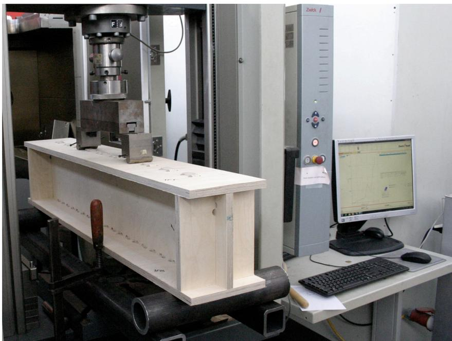
Fig 39. 4-point bending experiment setup.
