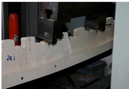
Fig 43. Failure mechanisms of the test samples. Sample 1A and 2A collapsed in a sequence of failure modes.
