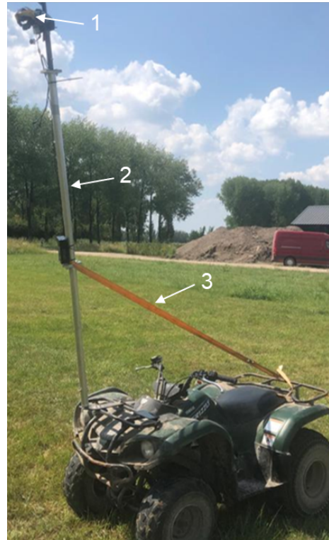
Figure 2: Experimental setup consisting of FLIR thermal camera (1) attached to a quad via aluminum bars (2) and a tension strap (3).
