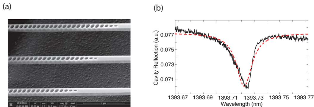
Fig. 2. (a) SEM image of fabricated nanophotonic devices. (b) Reflection spectrum of one of the devices with total Q factor  $\sim 100,000$ .
