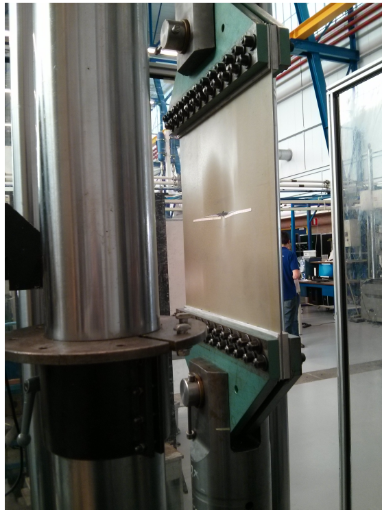
Figure D.3: Out of plane displacement observed during testing.
