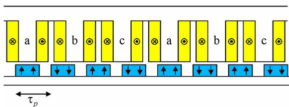
Figure 6: Linear permanent-magnet machine with concentrated coils.
