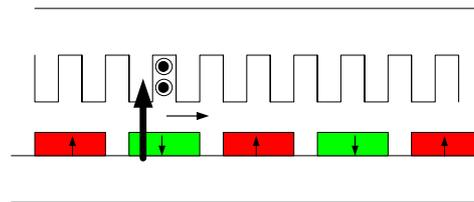
Figure 4: Electromagnetic forces in an electrical machine.
