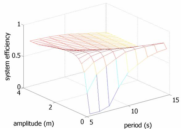
**Figure 4:** Average generator system efficiency (including cable and power electronic converter) as a function of wave height and wave period.
