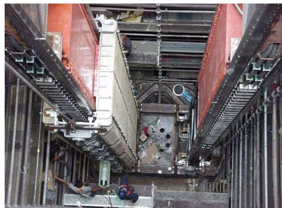
Figure 2: Photograph of the linear permanent-magnet generator in the AWS.
