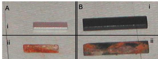
**Figure 8:** Alternative coatings for magnets (i) as new, (ii) after years submerged in sea water
