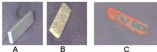
**Figure 7:** Standard coating for magnets (A) New, (B) after 6 weeks and (C) after 2 years submersion in seawater.
