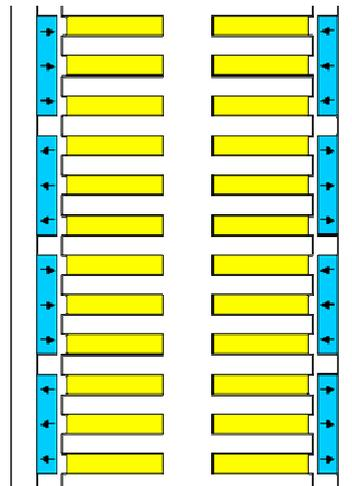
Figure 1: Sketch of a cross-section of the linear permanent-magnet generator of the AWS.
