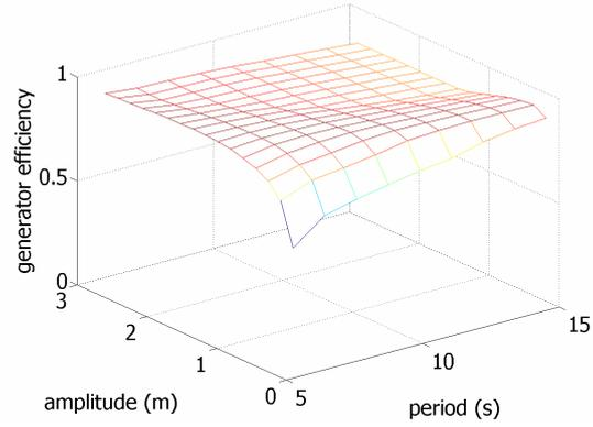
**Figure 3:** Average generator efficiency as a function of wave height and wave period.
