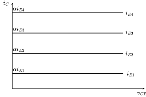
Figure 2.8: Theoretical collector current versus base collector voltage plot
