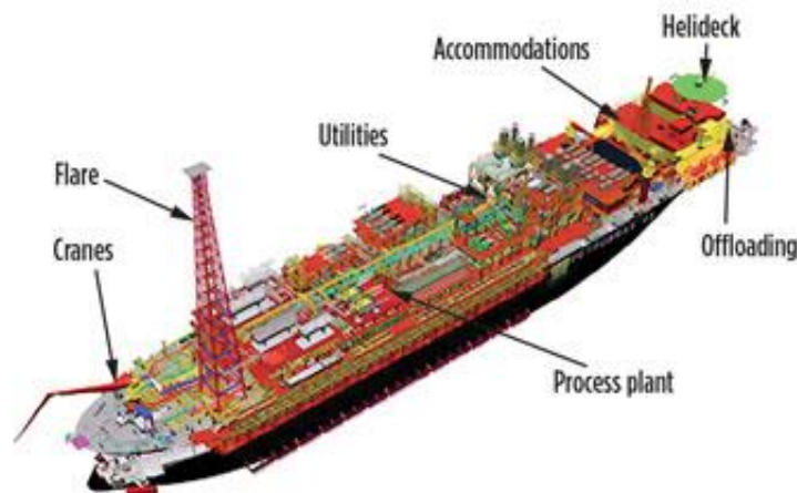
Figure 7: typical FPSO layout [9]
