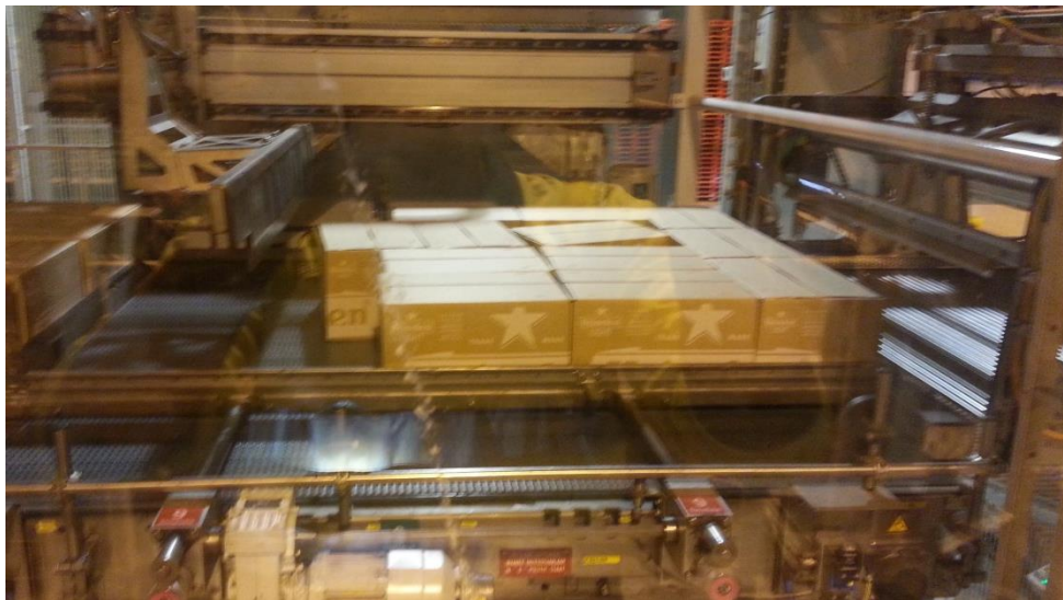
Figure 28 - Picture of blocked palletizer machine due to wrong pattern
