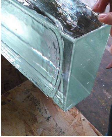
Glass frame for the Crystal Houses, produced by Vetreria Resanese, exhibiting deep lap marks. The improper flow of the molten glass at the bottom of the mould could be attributed to a non-sufficiently heated mould surface.
