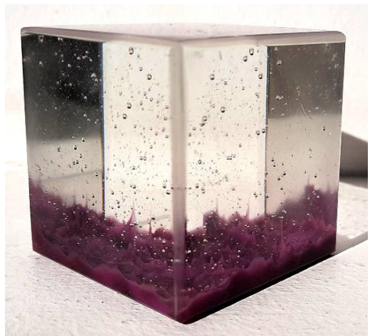
Fig. 1.1 The beauty of inhomogeneities in cast glass. 50mm cubic kiln cast specimens produced at TU Delft Glasslab from Leerdam crystal glass waste (left) and Bullseye art glass (right) at 870°C.
