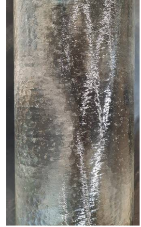
Cast glass column by John Lewis Glass Studio exhibiting an intense "orange peel" structure at its surface, due to contact with a non-sufficiently heated mould.
