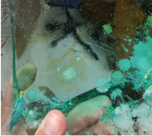
Piece of glass (ownership of J. Varner) retrieved from a glass furnace, showcasing the most common encountered melting defects such as devitrification stones, bubbles, cord and colour streaks.
