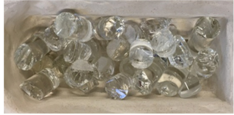
Placement of cullet (borosilicate rods by Schott) inside the investment mould, for the kiln-casting of the sample on the left.
