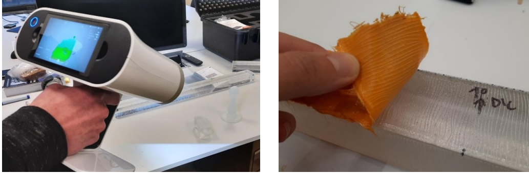
Fig. 8.1 Trials on documenting surface defects on cast glass prior to testing. Left: The 3D scanner Artec 3D Leo can be rotated around the object (volume capture zone 0.16\text{m}^3 ), producing a 3D point cloud of 0.1\text{mm} accuracy, yet renders inaccurate results in the case of glossy transparent materials, even if these are coated with an antiglare spray. Right: Replicas of cast glass surfaces – in combination with high-res photography- can be useful for tracing back to the fracture origin site, upon destructive testing. Polyvinylsiloxane, commonly used in dentistry as a fast-curing and highly accurate impression material, can effectively replicate scratches and indents found on the cast glass surface.
