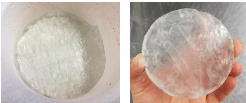
Fig.2.16 Czech glass cast at 950^\circ C . Post-processing is required to remove the shrinkage of the top surface and reveal the actual transparent glass.
