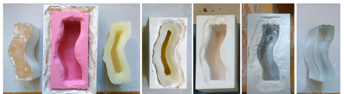
Figure 2 Production steps from MDF mould to final glass model
