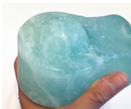
Fig. 2.15 Melting experiments with PPG furnace waste glass. (a) Green glass before (left) and after (right) casting at 860°C. (b) Aquamarine glass cast at 860°C (left) and 1200°C (right).
