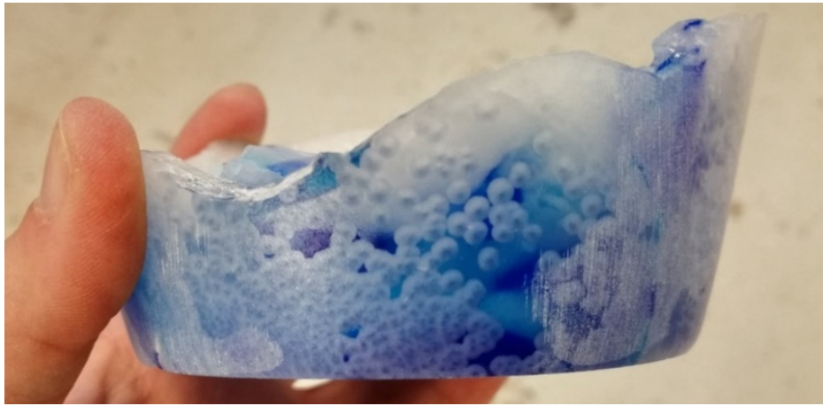
Fig. 2.10 Glass sample from the flowerpot used during the 860°C casting experiment, showing the formation of crystals.
