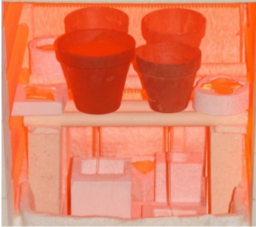
Fig. 1.14 Kiln-casting process followed at the TU Delft Glasslab: a viscous thread of glass slowly flows from the flowerpot down inside the mould as the kiln reaches the selected top temperature (left). The movement of the glass thread can be seen in the marks left on the glass-mould surface (right image shows the side view of the component, prior to polishing) but also in the cord present in the bulk of the glass component.
