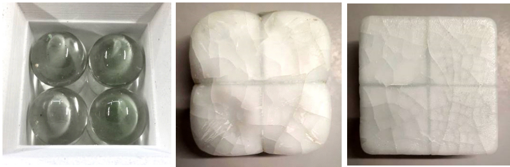
Fig. 1.30 Kiln-casting experiment at 970°C, using two layers of Ø25mm clear glass spheres introduced inside the investment mould (left). The top (middle) and bottom (right) aspect of the cast specimen suggest the equal filling of the mould space by each sphere.
