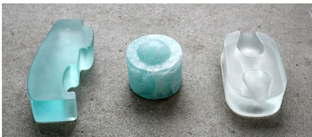
Fig. 2.13 PPG furnace waste aquamarine cast at 1120°C (left) and at 860°C (middle). PPG Starphire cast at 1120 °C (right).
