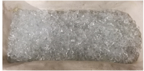
Cullet distribution inside the mould prior to casting the sample on the left.
