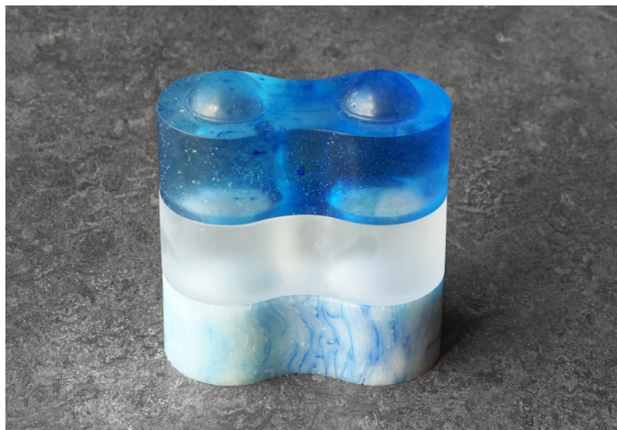
Fig. 2.8 Glass samples cast employing Sprucepine clear and blue glass waste (top and bottom) and lead crystal (middle element). The figure shows the effect of casting temperature to the structure of the glass component. Although the top and bottom sample are cast using the same glass, the one below, cast at 860°C crystallized, in comparison to the clear blue component on top, cast at 950°C.
