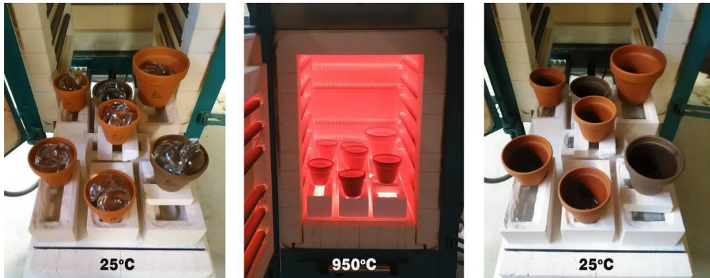
Fig. 1.29 Kiln-casting method followed at the TU Delft Glasslab, employing low temperatures/high kinematic glass viscosities that intensify the creation of casting defects in the glass.
