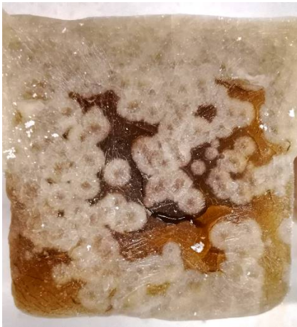
Surface crystallization developed along the side surface of a kiln-cast component, which was in contact with the silica-plaster investment mould (TU Delft Glasslab). The higher than usual alkali content (18% wt) and aluminium oxide (3.4 wt%) of this soda lime silica glass by Lamberts could be responsible for the extended reaction to the mould material.
