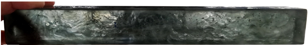
Fig. 3.7 “Lead CRT, 870°C” specimen containing intense cord (seen as wavy lines) and bubbles.
