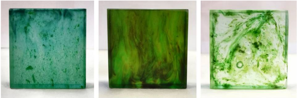
Fig. 1.28 Re 3 Glass prototypes kiln-cast at the TU Delft glass at 1120°C out of car windshields (left), containers (middle) and oven-doors (right). The remelting of commercial glass waste in its “as-received” form introduces a rich pallet of defects in the glass network. The severity of such flaws is uncertain.
