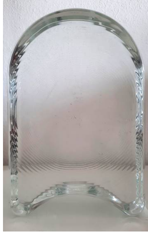
Pressed cast glass brick for the Atocha Memorial produced by Schott. Chill marks from the pressing process are evident at the top surface of the component.
