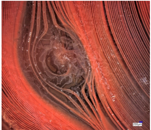
Fig. 1.15 Top surface of a kiln-cast specimen produced at the TU Delft Glasslab following the flowerpot method. The addition of colour helps tracing the spiral movement of glass while filling the mould (left). The spiral structure often overlaps with other structured layers -such as the crystallization film developed at the top surface- or gets interrupted by the uprising movement of bubbles (right).
