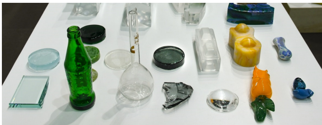
Fig. 2.26 Successful casting of pieces of (from left to right) float glass, bottle, laboratory tube, computer screen panel, lens, and mouth blown glass, demonstrating the numerous possibilities that arise in creating unique building components.
