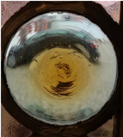
Bullseye window piece, Kloster in Trier, Germany. This is the centrepiece of crown glass, a hand-made flat glass produced by spinning a bowl-shaped blown piece of glass. Memory of this centrifugal action can be seen in the spiral cord, which is dominant in the piece.
