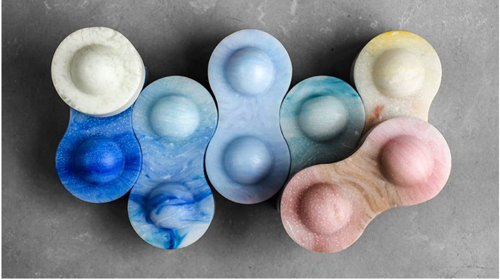
Fig. 1.27 Prototype for the Re 3 Glass project, kiln-cast at the TU Delft Glasslab. The interlocking building components are cast out of waste artware glass. The kiln-casting at a low temperature, below the liquidus point of this glass (870°C), and the slow cooling lead to the partial crystallization of the glass, and thus marble like appearance of the components.
