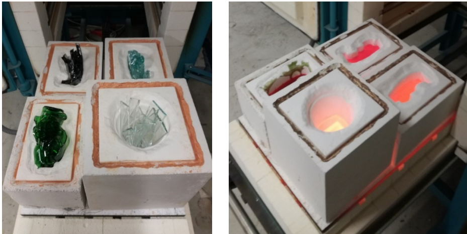
Fig. 2.4 Kiln-casting experiment at 1120°C, portraying the differences in luminosity among the various coloured samples.
